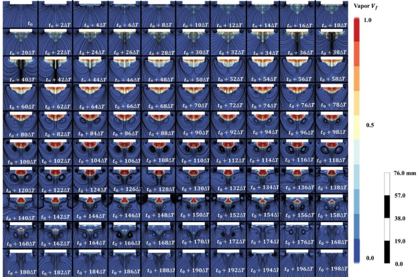
Figure 6.9: A series of vapor volume fraction contour plots that demonstrate a single cycle of the growth and collapse of acoustic cavitation under a 16 mm horn tip diameter. Surface streamline and vector plots were also highlighted in the contour plots to visualize the proximal flow behavior and direction.
