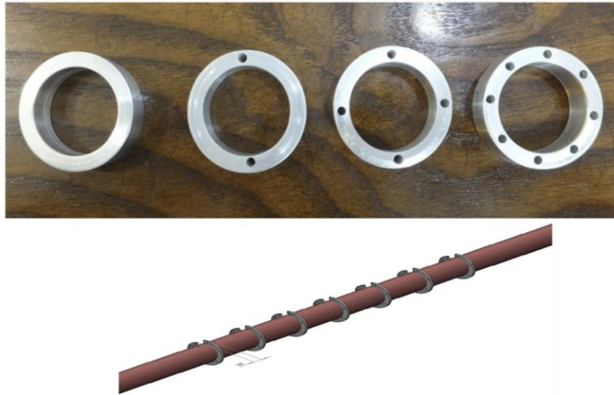
Figure 2.5: Discontinuous perforated rings and helical turbulators proposed by Sheikholeslami et al. [8], [9]
