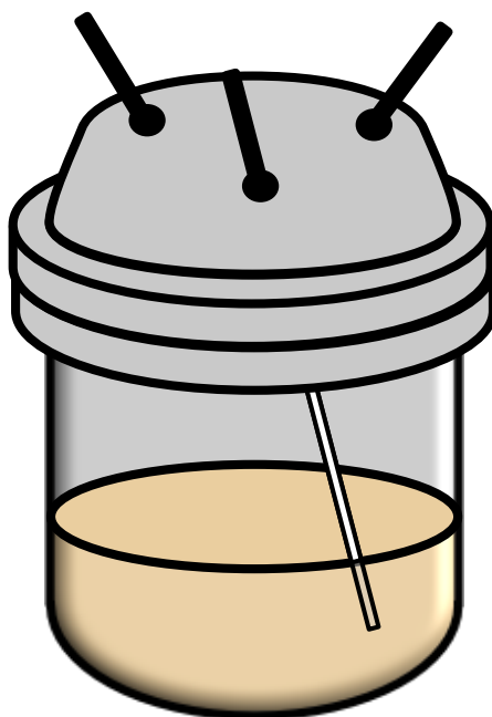
Figure 4.5: The suspension reactor, fitted with PTFE tubing from the carrier gas input into the solution, leading to the solution to decrease purging time.
