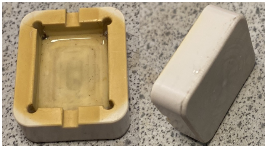
Figure 4.10: The PEEK insert after approximately 10 photocatalytic reactions (20 - 30 hours UV exposure) on the top (left), which is exposed to UV and houses the photocatalyst. This picture is taken after washing with soapy water, acetone, hexane, petroleum ether and sonication to ensure discoloration is not an adsorbate. Rear and side view (right), which is not exposed to any UV, due to being housed inside a stainless steel cavity. The top side shows color change indicating UV induced degradation.
