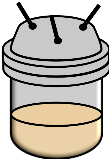
Figure 4.2: A suspension reactor, in which the suspension of photocatalyst in water and methanol (yellow) is stirred and irradiated from the side. The lid is fitted with 3 Swagelok joints for 2 inputs of carrier gas, and one output to carry products to the GC. The lid is screwed on and sealed by 2 rubber toric joints.
