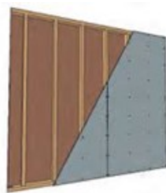
Figure 2.28: Wall constructive solution for standard dwelling (baseline).
