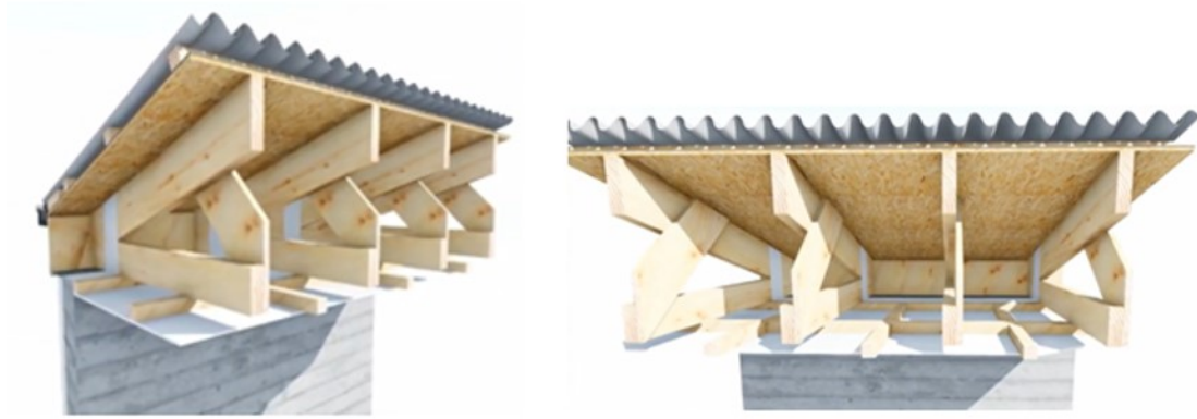
Figure 2.27: Roof constructive solution for standard dwelling (baseline)[141].
