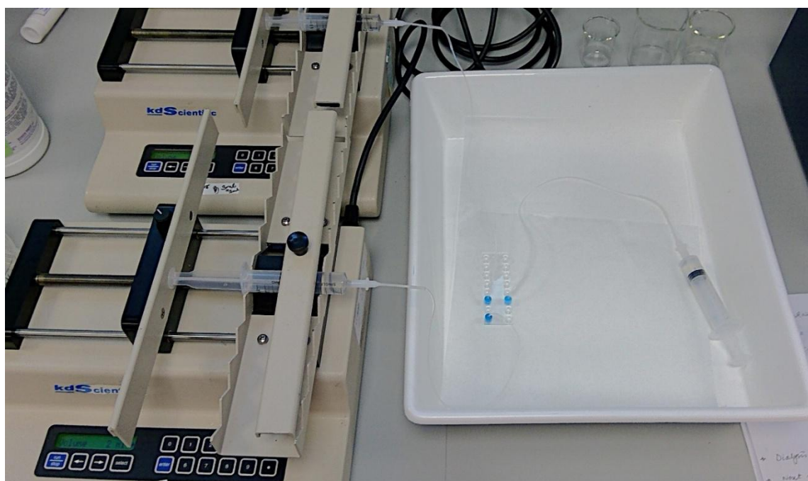
Figure 1: Visual representation of the staggered herringbone mixing set-up to produce LNPs. One pump for each of the two phases in the LNP production. Together they were set to dispense in a 3:1 ratio of aqueous: organic phase.
