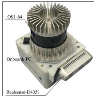
Figure 2-13. Example hardware setup for vision-LiDAR fusion used in the Newer College dataset [104]. This configuration includes an Ouster OS1-64 3D LiDAR sensor and an Intel RealSense D435i RGB-D camera.
