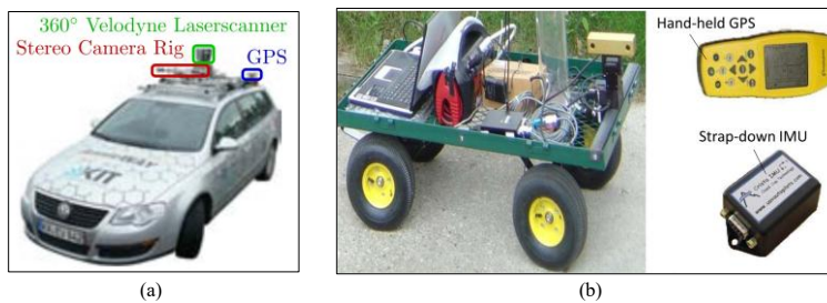
Figure 2-28. Examples of hardware setups used for acquiring ground truth trajectories of mobile platforms in SLAM benchmarks. (a) Hardware configuration used for data collection in the KITTI dataset [96]. In this setup, an OXTS RT 3003 localization system—comprising GPS, GLONASS, an IMU, and RTK correction signals—is employed to determine the platform's ground truth trajectory. The figure explicitly indicates only the GPS component, omitting annotations for the other devices. (b) Hardware configuration used by Abdallah et al. [137], featuring a handheld GPS unit and a strap-down IMU to acquire the ground truth trajectory of the mobile platform.
