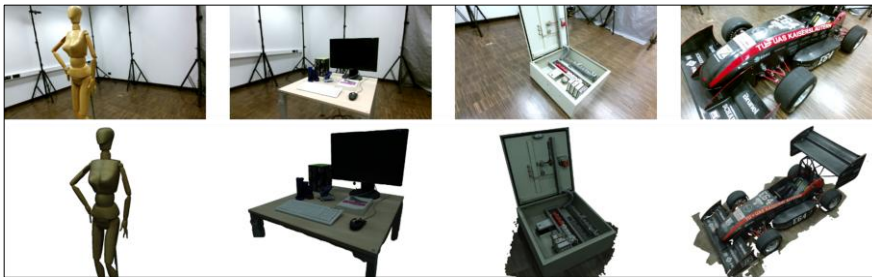
Figure 2-32. Objects and their reconstructed 3D geometries from the CoRBS dataset [108], used as a benchmark for evaluating mapping performance. Top: The objects used in the CoRBS dataset for mapping benchmark. Bottom: The corresponding reconstructed ground truth geometries of the objects shown in the top row.
