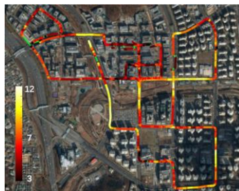
Figure 2-27. Scalar field visualization of GNSS signal intensity along the route used for data collection in a complex urban outdoor environment (Liu et al. [139]). Yellow segments indicate areas with strong GNSS signals, red segments indicate areas with weak GNSS signals, and green segments represent areas where GNSS signals are entirely unavailable. As illustrated, GNSS signals are frequently disrupted, with areas of weak or no signal significantly outnumbering areas with strong signal reception. This demonstrates that in urban environments, GNSS performance is inevitably impacted by high-rise buildings.
