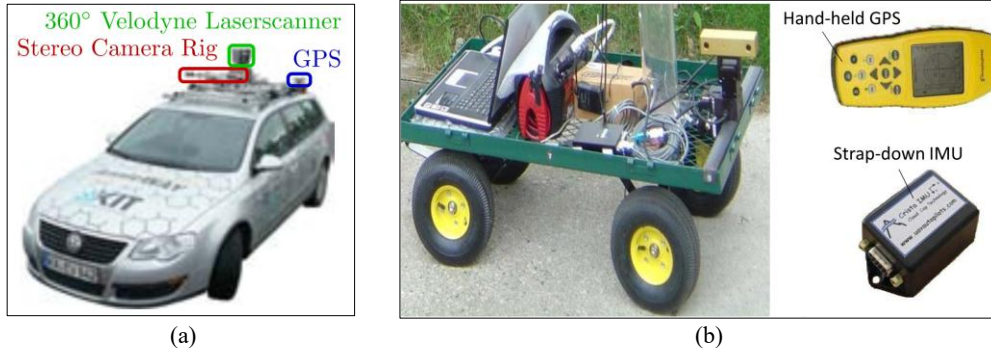
Figure 2-28. Examples of hardware setups used for acquiring ground truth trajectories of mobile platforms in SLAM benchmarks. (a) Hardware configuration used for data collection in the KITTI dataset [96]. (b) Hardware configuration used by Abdallah et al. [137].
