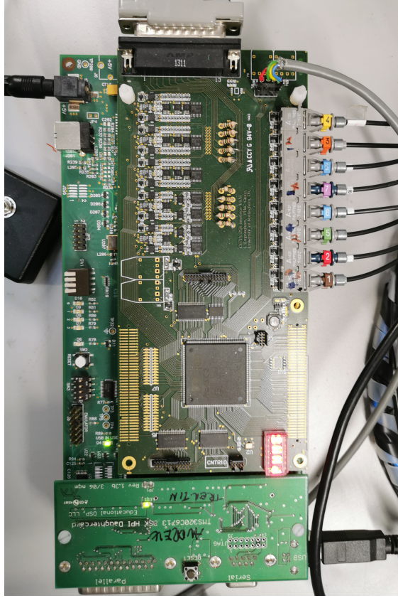
Figure 6.1: Buck Converter Digital Signal Processing Board
