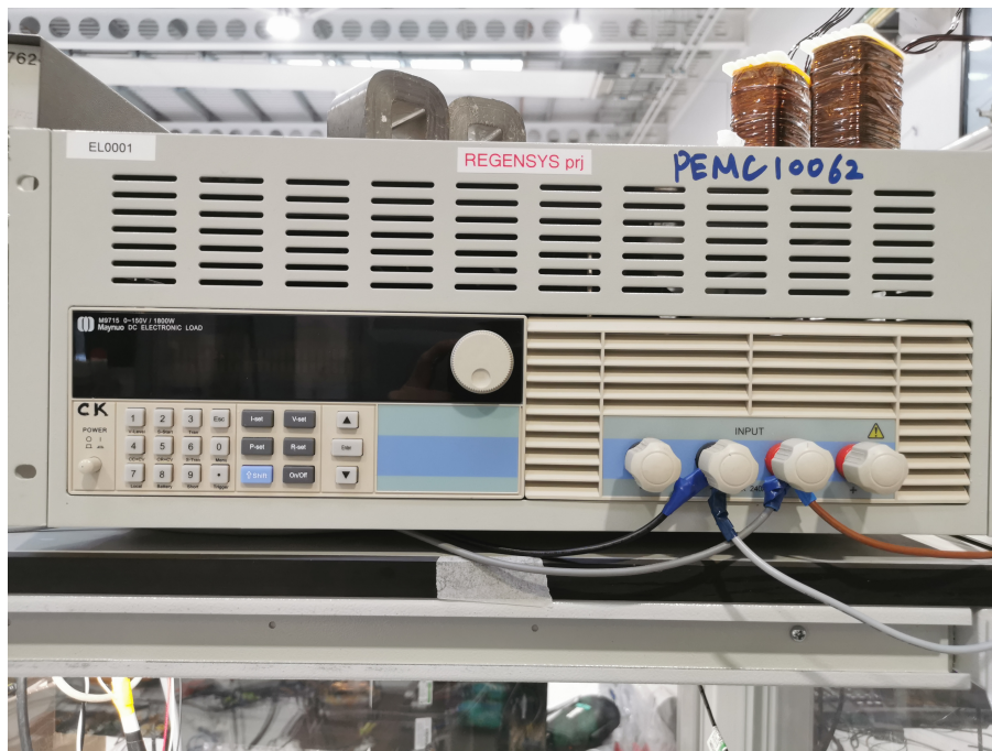
Figure 6.8: Interleaved Buck Converter Programmable Load
