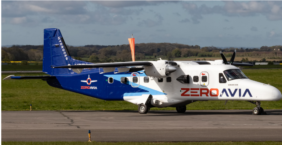
Figure 3.2: Do28NG Hydrogen Propulsion Test Bed [95]
