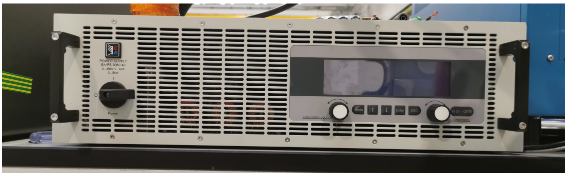
Figure 6.4: 5 kW Power Supply Unit for the DC Bus
