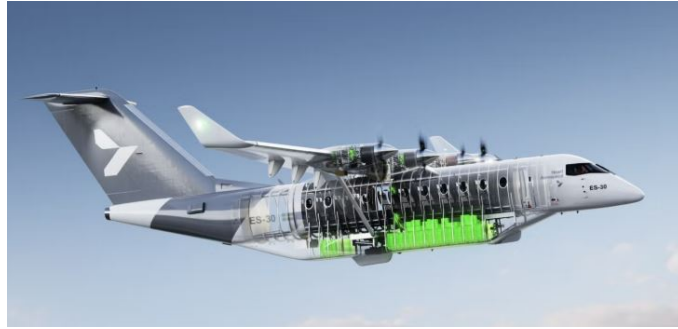
Figure 2.9: Hart Aerospace battery location proposal
