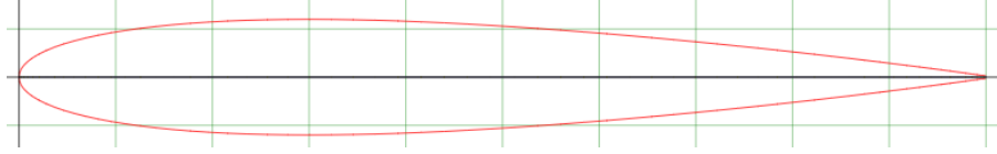
Figure 2.13: NACA 0012 Airfoil for Cessna 175 Horizontal Stabiliser
