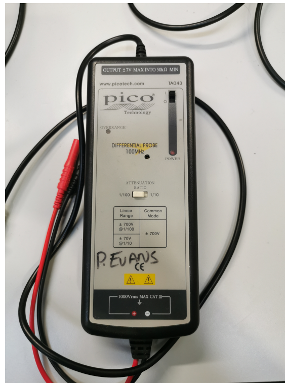
Figure 6.5: Differential Voltage Probe
