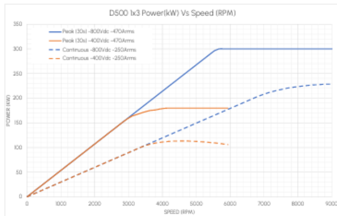
Fig3. The Evolito D500 achieves a continuous 230 kW and up to 300kW during peak testing conditions. This industry leading product offering is breaking conventional radial limits, boasting greater than 10kW/Kg+.
