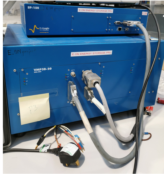
Figure 4.14: University of Nottingham's Galvano Electrochemical Impedance Spectroscopy Equipment
