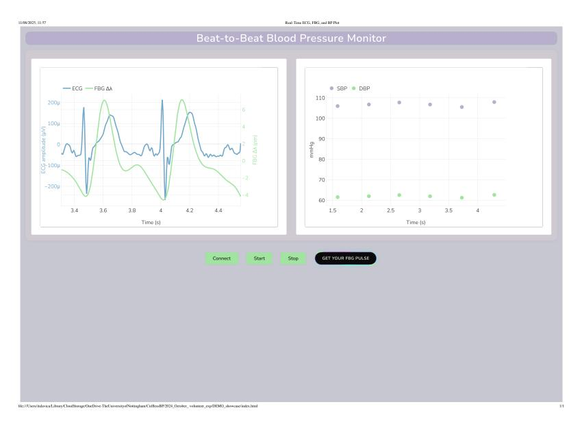
**Figure 3.17:** Web application for Beat-to-Beat BP measurement using PAT. Left Plot shows ECG and FBG waveforms, and the right plot shows the SBP and DBP derived from PAT using Gaussian Process Regression Model.
