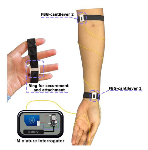
**Figure 3.2:** Arterial pulse measurement at wrist and upper arm with FBG-cantilever sensors.
