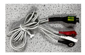
**Figure A.3:** ECG leads fabricated with Hirose connector, positive electrode (red), common electrode (white), DLR (black).
