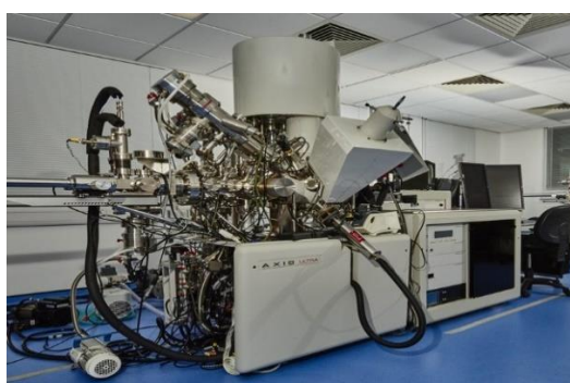
Figure 3. 7 The Kratos LiPPS instrument used for XPS.
