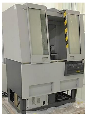
Figure 3. 6 PaNalytical X'pert Pro diffractometer used for XRD.
