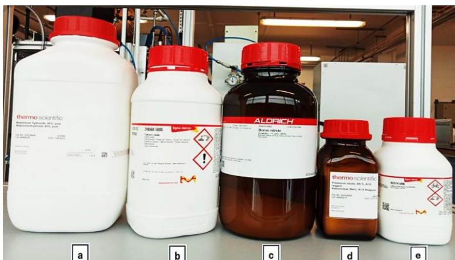
Figure 3. 1 A photograph showing the core TCES materials and dopants used: (a) \text{Mg}(\text{OH})_2 , (b) \text{Ca}(\text{OH})_2 , (c) BN, (d) \text{KNO}_3 , and (e) \text{LiOH} .
