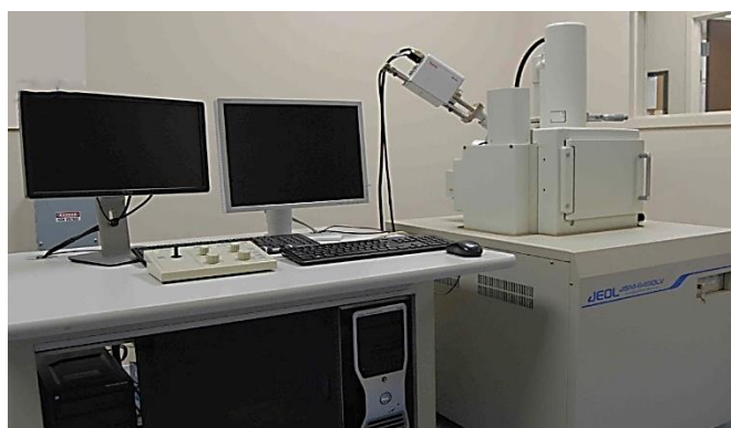
Figure 3. 9 JEOL 6490LV instrument used for SEM and EDX.
