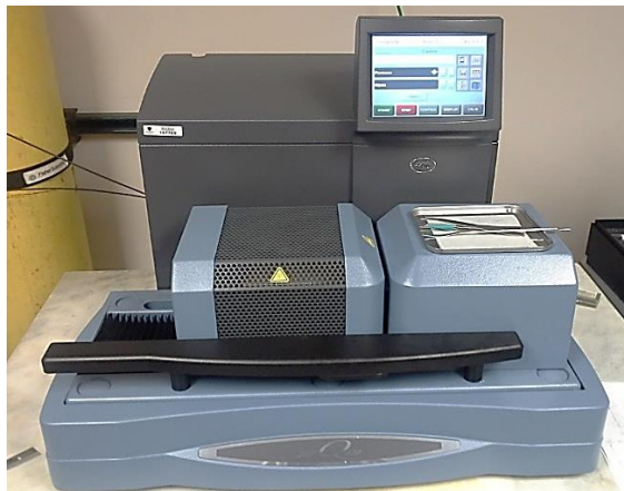
Figure 3. 10 SDT simultaneous DSC/TGA instrument used for DSC and TGA.
