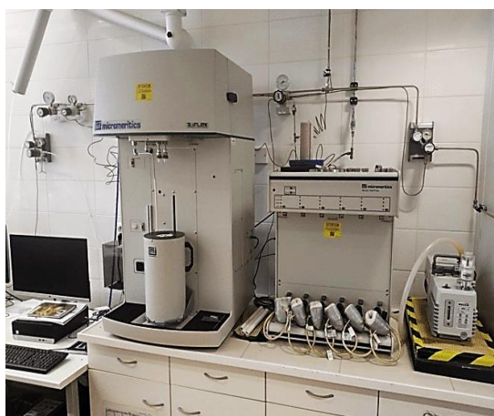
Figure 3. 8 The Micromeritics 3Flex analyzer used for BET analysis.
