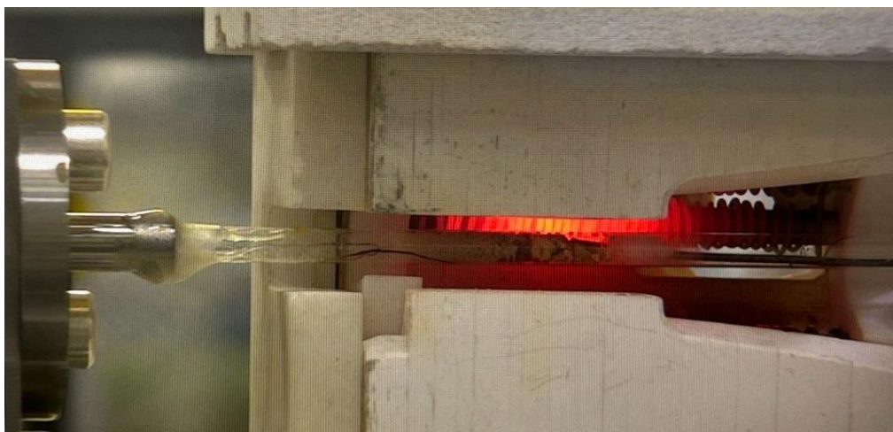
Figure 6.8. A picture of the experimental set-up for conducting operando EXAFS at Diamond Light Source. The sample is inside a quartz tube, and pictured next to the heating element.
