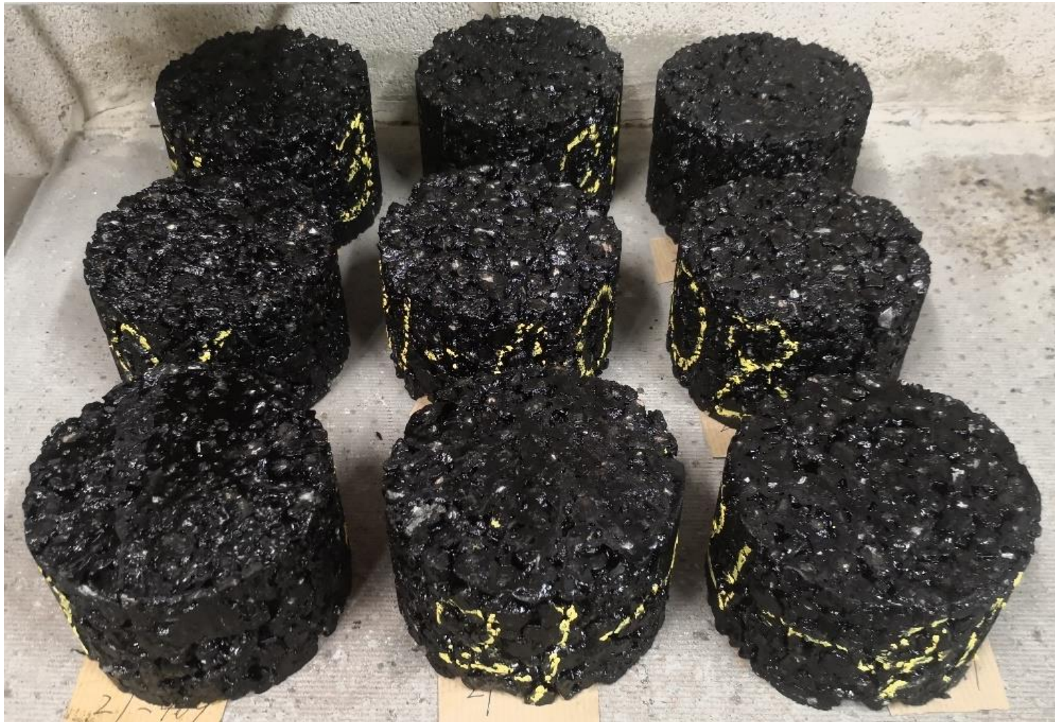
Figure 21: Cylindrical Asphalt Specimens Manufactured via the Marshall Method
