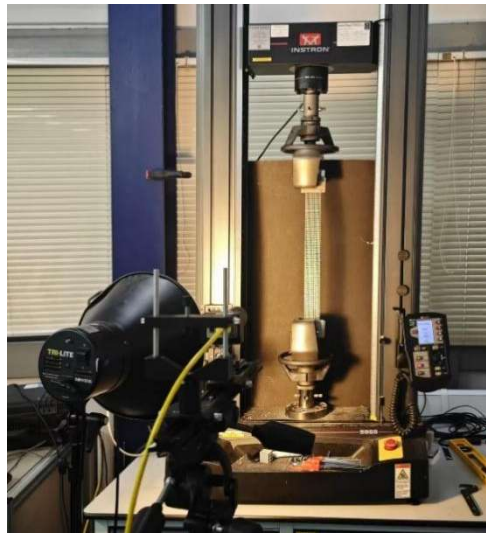
Fig. 7.6. Test setup of tensile tests on the UHTSS textile.
