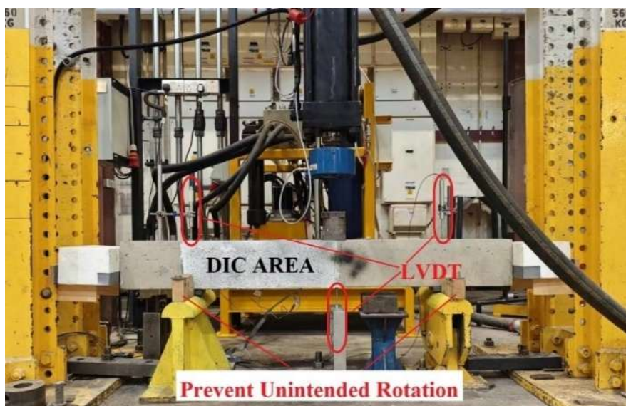
Fig. 4.1 Three-point bending test set-up of beams.
