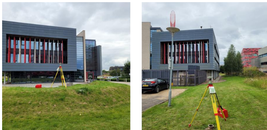
Figure 5.16 The GNSS receiver, antenna, collecting GNSS data on NGB11 (left) and NGB9 (right), which are front and behind NGB building, respectively.
