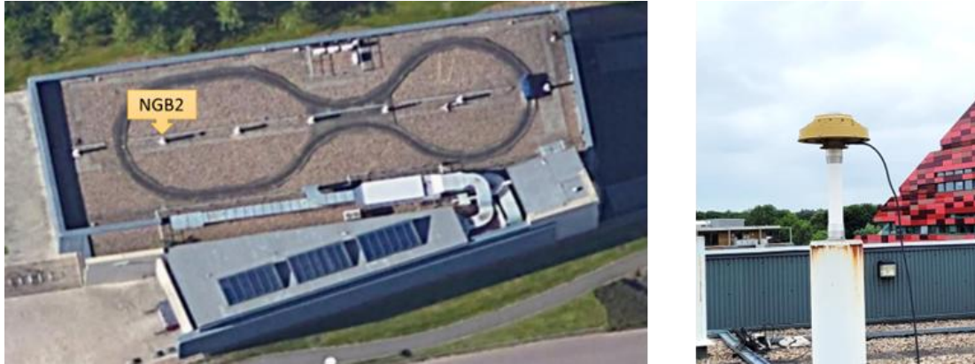
Figure 5.2 (left) View at the roof of NGI building, with the location of control point NGB2 and (right) the GNSS antenna installed on the top of the pillar of NGB2 [150].
