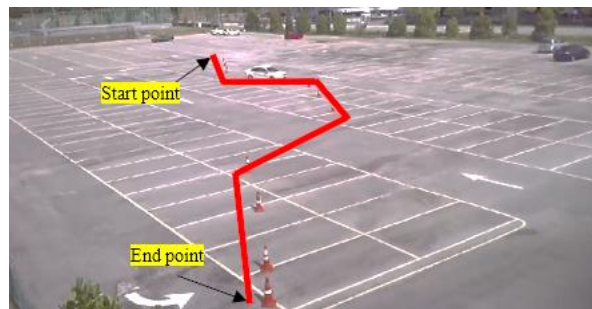
Figure 4-12 Double Lane Change field test
