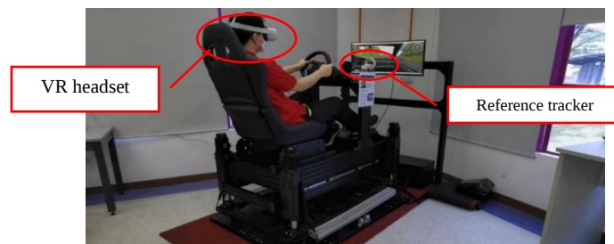
Figure 5-22 Virtual autonomous vehicle simulator with virtual reality and motion simulator.
