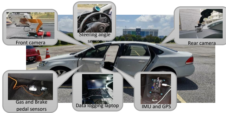
Figure 4-1 Sensor configuration of the instrumented vehicle
