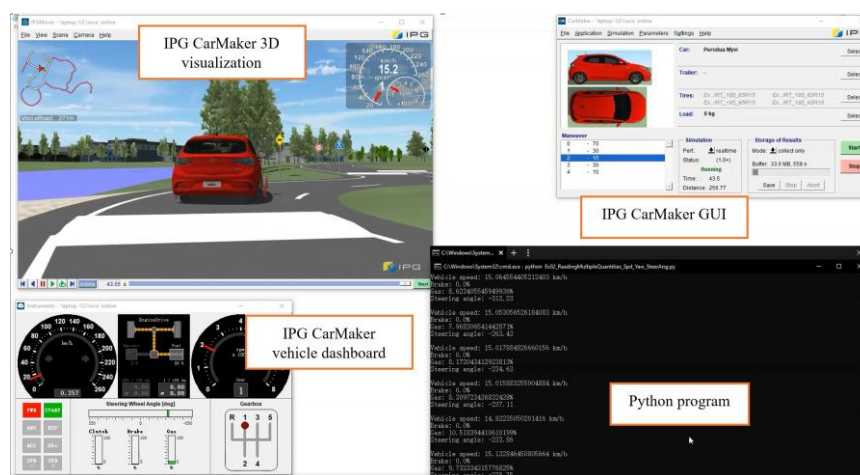
Figure 5-7 Reading vehicle speed, brake pedal, gas pedal and steering angle quantities from IPG CarMaker using Python.
