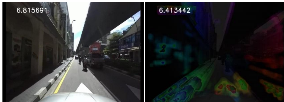
Figure 6-27 Estimated vehicle speed(left) and combined output with optical flow frame overlay(right).
