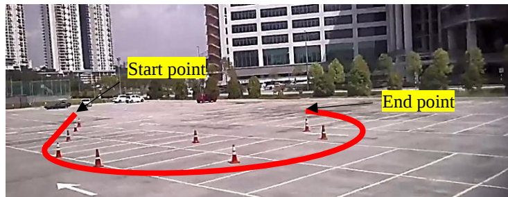
Figure 4-14 Step steer field test
