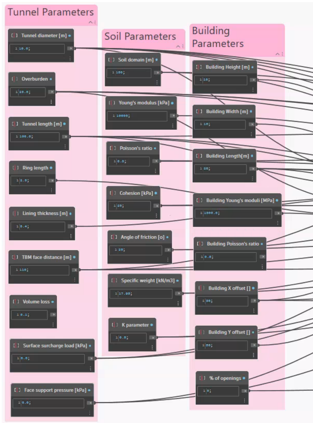
Figure B.1: Nodes describing the input parameters (identified from the pink background in Dynamo) for the tunnel, soil and building including the additional geometry-related parameters.
