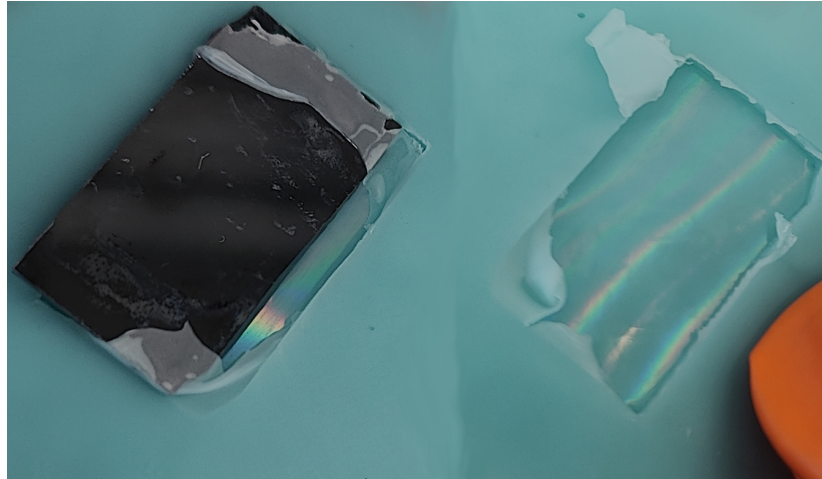
Figure 6.13: Pattern Transferred to Silicone from Si Mould
