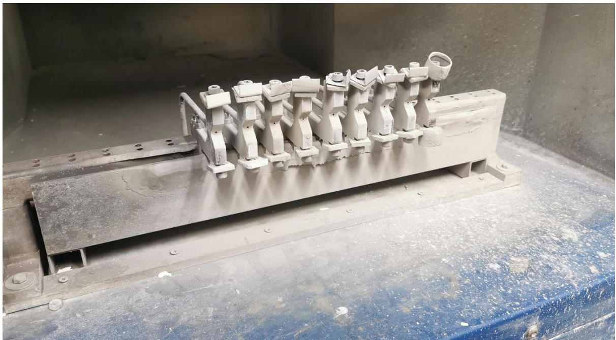
Figure 18. The substrate clamps and integrated cooling channels. For reference, the beam to which the clamps are mounted is 100 mm in length.
