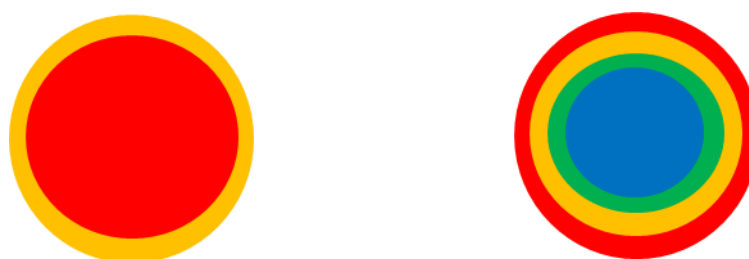
Figure 1.10 - Temperature profile of volumetric heating (left) compared with conventional heating (right).
