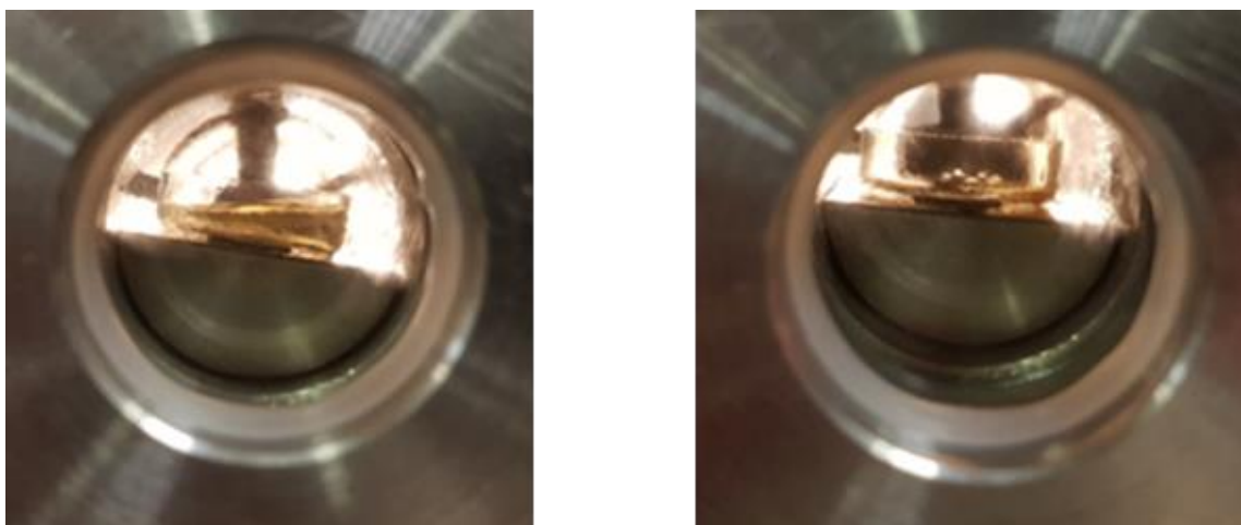
Figure 5.13 – Solubility test of a TBD-methanol solution in scCO_2 . The solution is clearly insoluble in CO_2 of pressure 55 bar at room temperature (left) but was seen to be fully soluble in scCO_2 at 172 bar and 85 °C (right).
