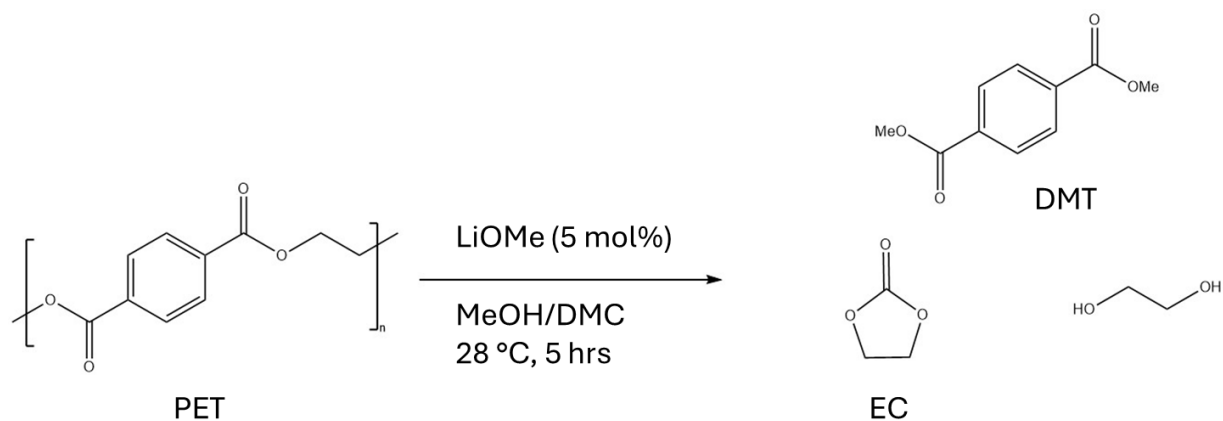
Figure 5.3 – Scheme of methanolysis procedure described by Tanaka 5 , the formation of ethylene carbonate (EC) by a secondary reaction between ethylene glycol and dimethyl carbonate prevents the backwards reaction, favouring PET depolymerisation.
