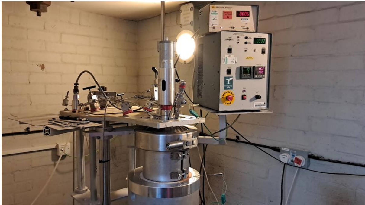
Figure 4.5 – Image of the 1 litre high-pressure autoclave scaled up impregnation experiments were conducted in.
