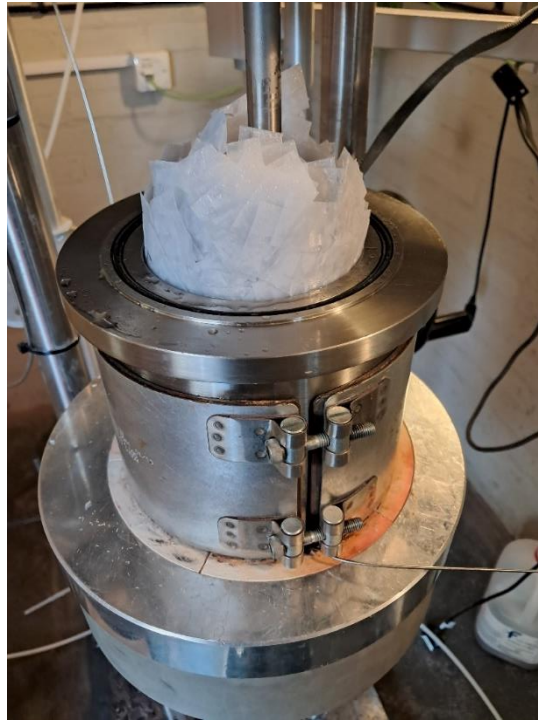
Figure 4.11 – PET impregnated with ethylene glycol immediately post scCO 2 impregnation.
