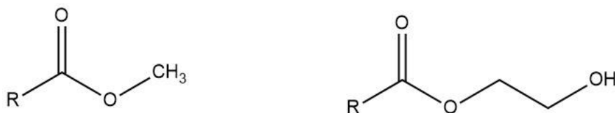
Figure 5.32 -The only two types of end groups seen in the PET methanolysis products. The ester functional group of DMT (left) and the alcoholic functional group derived from ethylene glycol (right).
