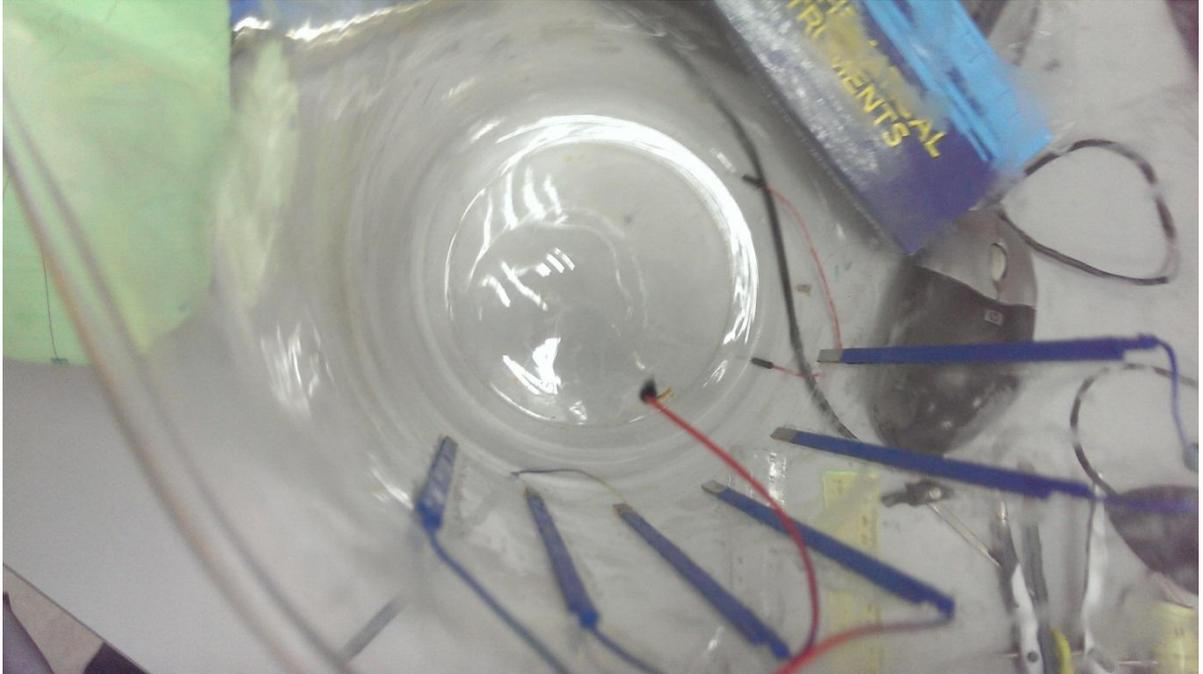
Attaching the copper electrodes to the beaker.
