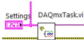
This VI creates a virtual channel to measure voltage and configure the sampling clock. The “Settings” is clustered with channels parameters which are passed from the UI.
