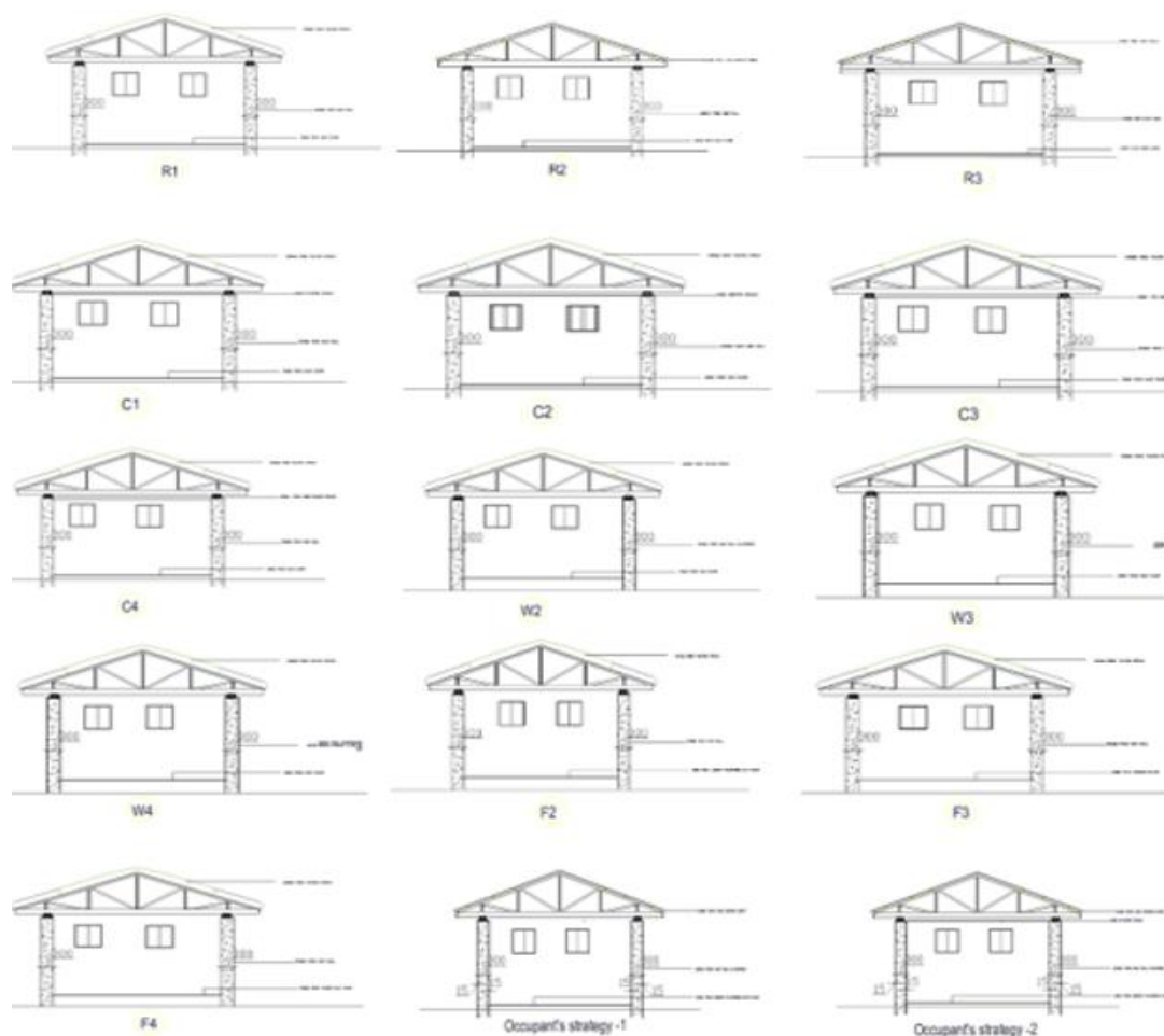
Figure 7-5: Potential arrangement of structural elements of Ilorin traditional adobe buildings
