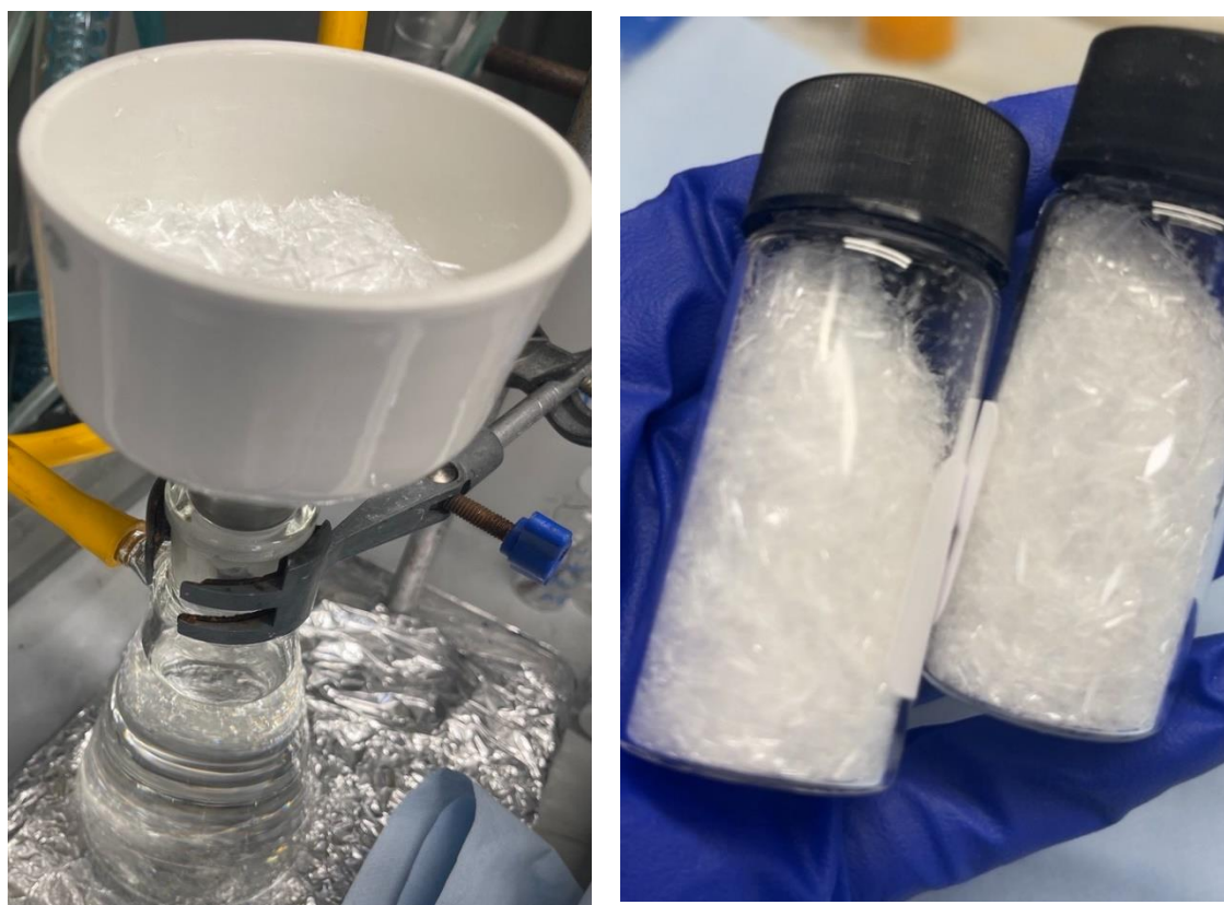
Figure 9. Purification of TBAPF 6 .
