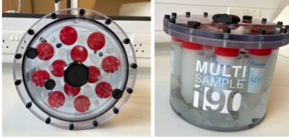
Figure 4.1 The phantom picture. The MultiSample 190F from Gold Standard Phantoms contains twelve 50 ml Falcon tubes filled with a range of glass bubble volume fractions from 0 to 2% in hydroxyethylcellulose gel.
