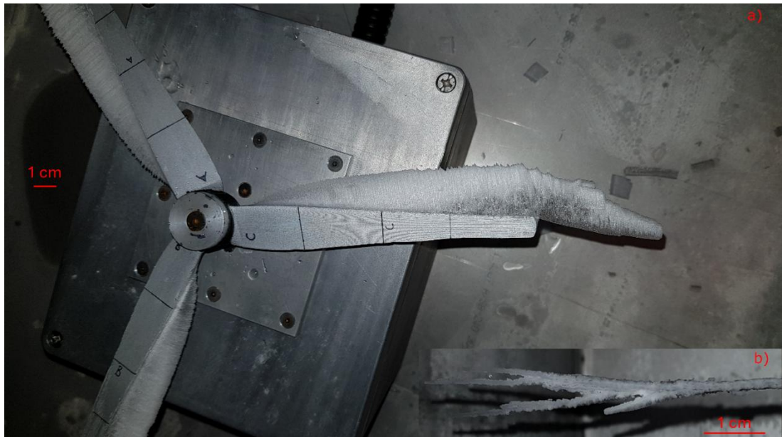
Figure 5.21 a) A plan view and b) tip growth viewed from the leading edge formed after 15 minutes at 500 rpm in a -4^{\circ}\text{C} environment.
