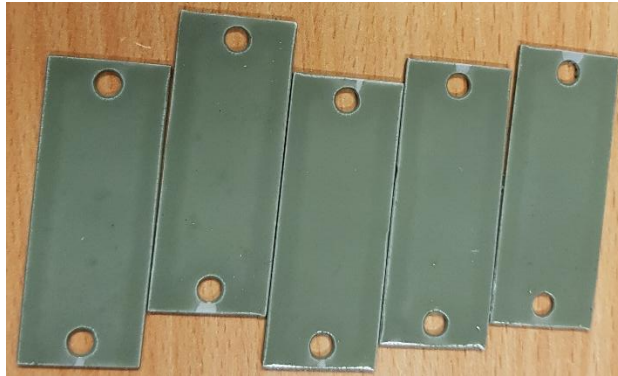
Figure 4.4 Colour gradient over the surface of 10% SiC in PDMS where darker regions near the edges are raised due to the surface tension dictating the distribution of the uncured polymer. Substrates are 20 mm x 50 mm.
