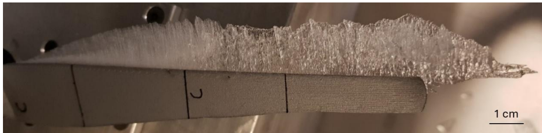
Figure 5.20 An example of the ice transitioning from rime to glaze down the blade. 500 rpm, -2^{\circ}\text{C} , 15 minutes.
