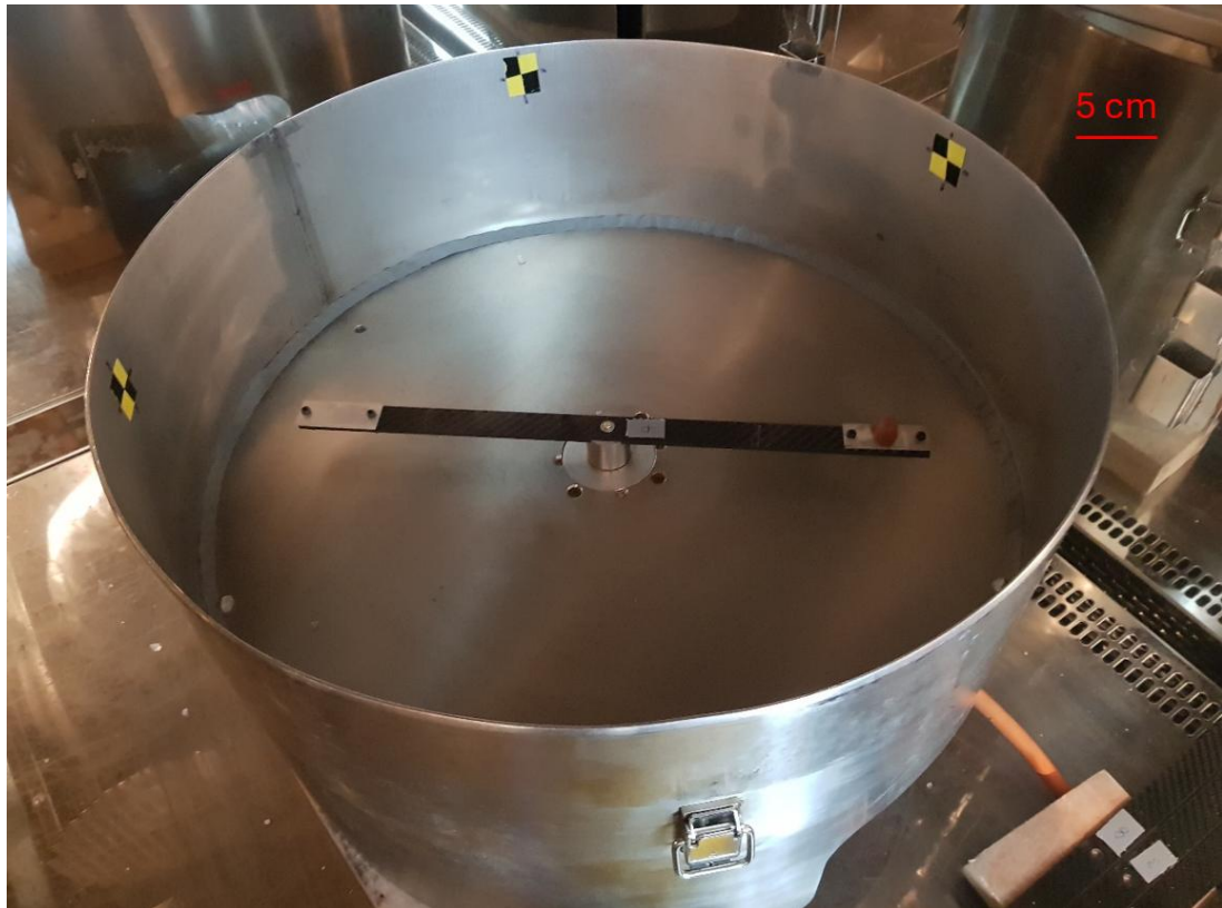
Figure 4.24 Image of the steel drum and rotating arm used in the CAT.
