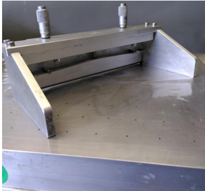
Figure 4.2 Blade with an adjustable height that works with the film applicator to spread material by being pushed over the substrates covered in an excess of the uncured polymer. Pictured atop the Film applicator table in Figure 4.1.
