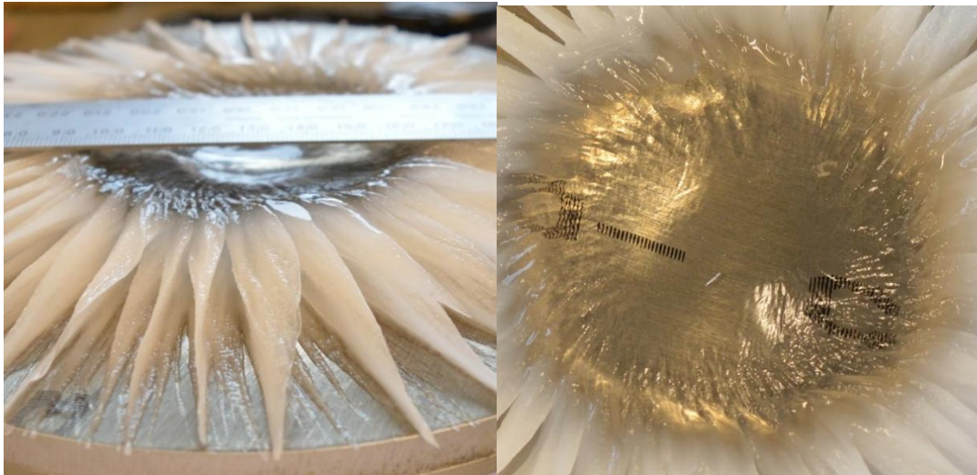
Figure S PDMS disc, from two perspectives, with the centre covered with glaze ice that is much thinner than at the transition point containing ripples with a much smaller wavelength than the protrusions.
