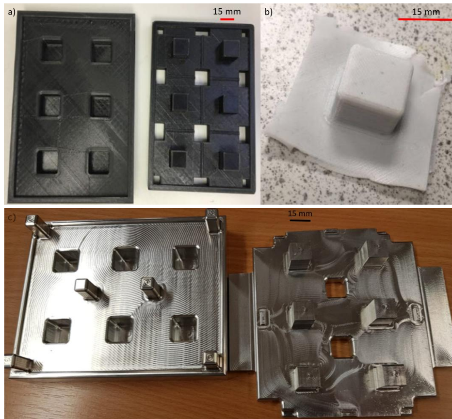
Figure 4.15 a) 3D printed prototype for a mould to make 15 mm ice cube moulds that formed 15 mm ice cubes. b) a mould produced by the prototype with large wings around the cube itself to facilitate its delicate removal. c) the final mould machined from an aluminium block.
