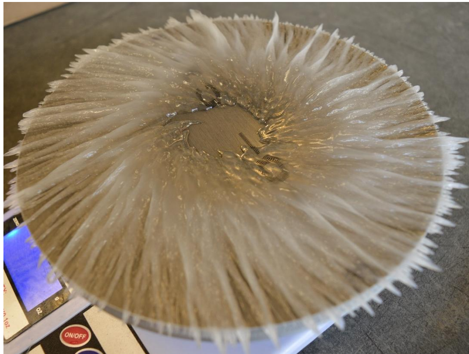
Figure R PDMS coated disc with no accretion forming at the centre.
