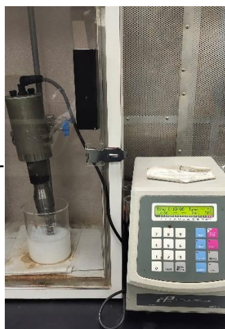
Ultrasonic treatment to disperse aggregates
