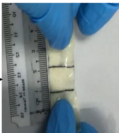
S_r of the smart rubber was initiated and \epsilon_r was measured
