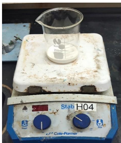
Continuous stirring of the rubber mixture at 200rpm for 60 minutes at room temperature
