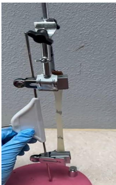
Rubber film was secured on the modified special elongation device
