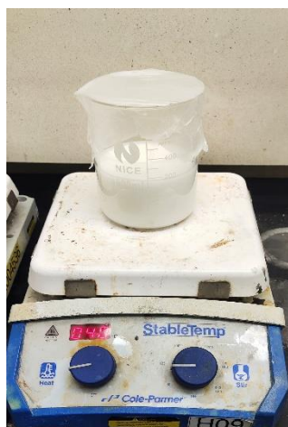
Mechanical stirring of the mixture at 40°C, 100 rpm
