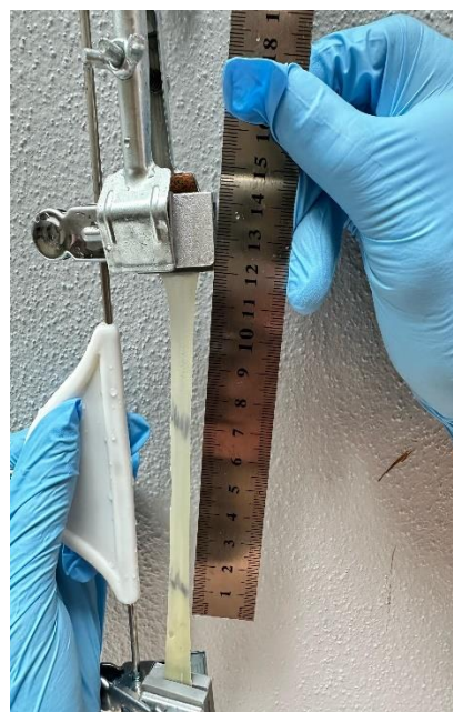
The rubber film was elongated to 600% strain
