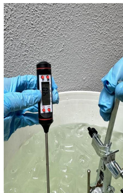
Rubber film was quenched in 4 °C ice water
