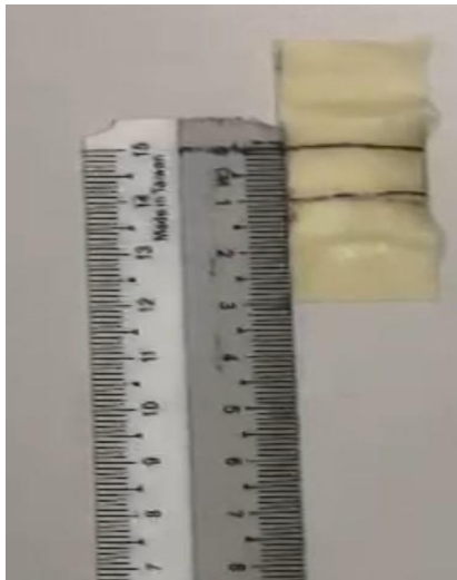
Initial gap of smart rubber film was indicated as 1cm
