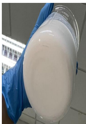
Visible aggregates were completely dispersed
