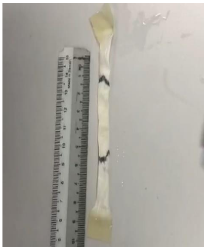
Smart rubber film unloaded from clipper and \epsilon_f was recorded
