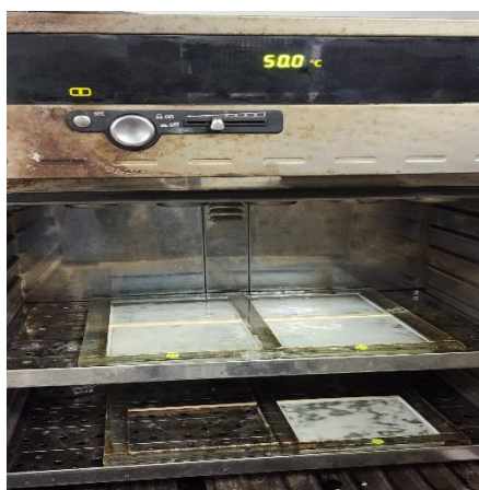
Rubber specimen was heated at 50 °C for 5 hours
