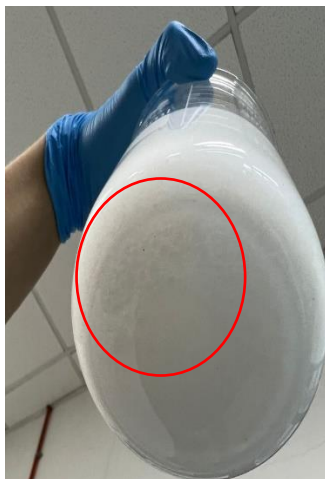
Visible aggregates after centrifugations
