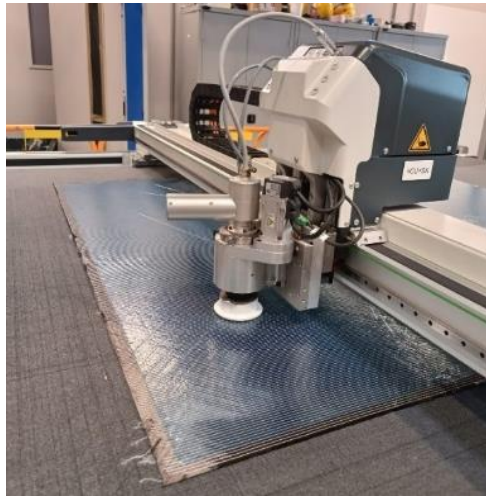
Figure 3.5. Automated cutting machine, X-CUT-TT, cutting the NCF samples to the required size.
