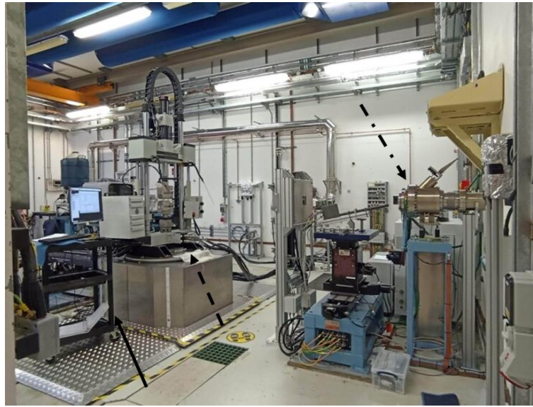
Figure 3.11. Overview of the EH1 in the I12 beamline at the Diamond Light Source facility. The x-ray source is provided into the hutch by the source indicated by the dash-dot arrow; the table with the testing machine, for the tensile test, is pointed out by the dash arrow; the data obtained during the mechanical testing were collected by the computer indicated by the continuous arrow, and transmitted to a computer into the control room so that data could be monitored and analysed in real time
