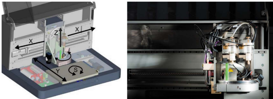
Figure 4.1: Diagram of the motion systems (left), modified from [273], and photograph (right) of the PixDRO LP50 printer.
