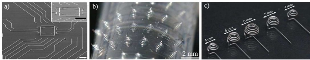
Figure 2.8: Direct ink writing of conductive metals in 3D shown in (a) an SEM image of InGa 3D circuitry, both scale bars = 100 \mu\text{m} , reproduced from [137], and optical images of helical antennas made from (b) laser-sintered silver, reproduced from [135], and (c) Field's metal, reproduced from [136].
