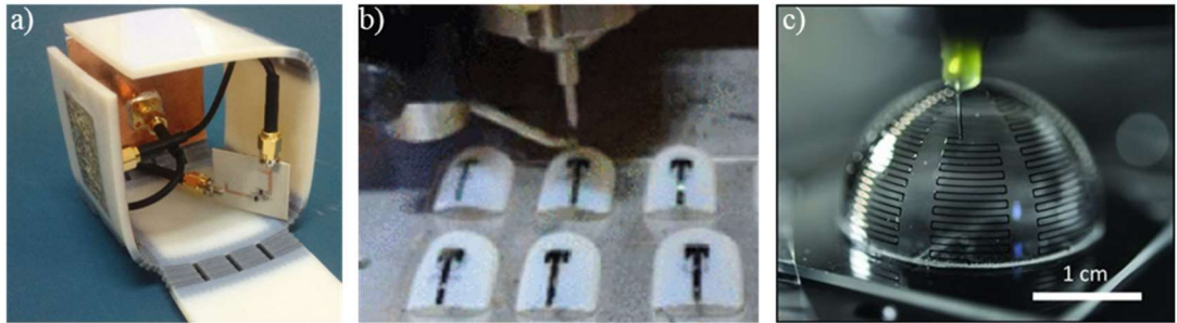
Figure 2.13: Optical images of antennas produced by (a) IJP silver patch antennas onto an inkjet-printed shape-memory polymer, reproduced from [71], (b) aerosol jetting silver onto acrylic nails for identification antennas, reproduced from [185], and (c) direct ink writing silver onto a glass hemisphere to create an electrically small L band antennas, reproduced from [187].
