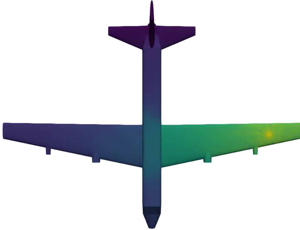
Figure 9: Point-force excitation of a simple aircraft mesh simulated using DEA with N_b = N_\beta = 5 , which corresponds to two boundary elements per edge of the triangular mesh elements. The colour scale shows the calculated energy density and runs from low energy (dark blue) to high energy (yellow).
