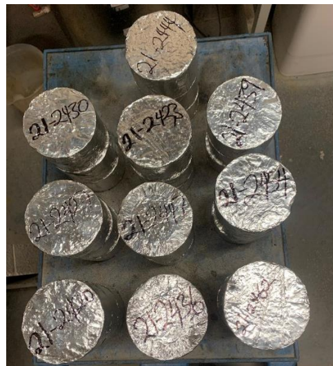
Figure 3-69: Foil-sealed asphalt specimen prepared for bulk density and air void content determination using the sealed specimen method.
