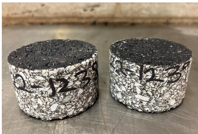
Figure 6-119: Cores drilled from filled potholes for the estimation of AVC.
