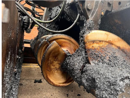
Figure 2-42: Illustration of an auger in an asphalt paver, captured on site after paving works.
