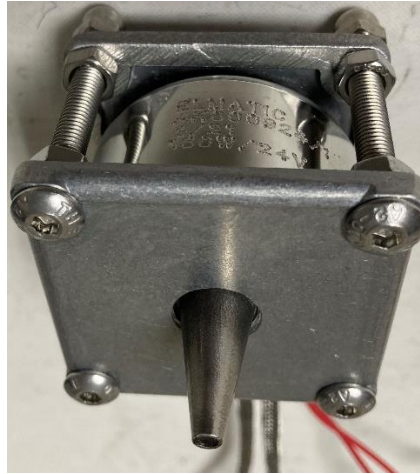
Figure 4-76: The assembled 24 V, 150 W heating chamber.
