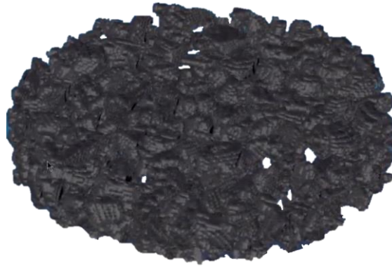
Figure 5-99: An illustration of loose coarse aggregates (> 2 mm) coated with mastic (fines, filler and bitumen mixed) from the physics engine simulation.
