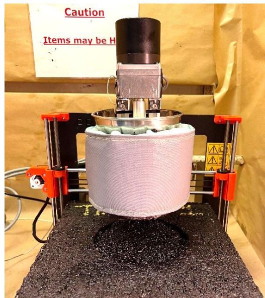
Figure 6-110: The complete APFM setup at NTEC during the pothole filling process. Electric motor torque represents the rotational force generated by the motor. The maximum power was approximated through a speed-torque optimisation, resulting in the largest area beneath the speed-torque curve.
