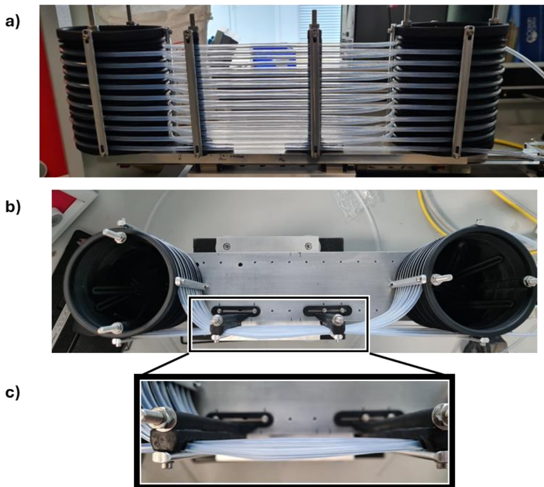
Figure 6.07: Images of the assembled KRAIC-S v2 on the translation stage with a) front on view, b) top down view, and c) view of top-down X-ray analysis region with bowing tubing on every return loop.
