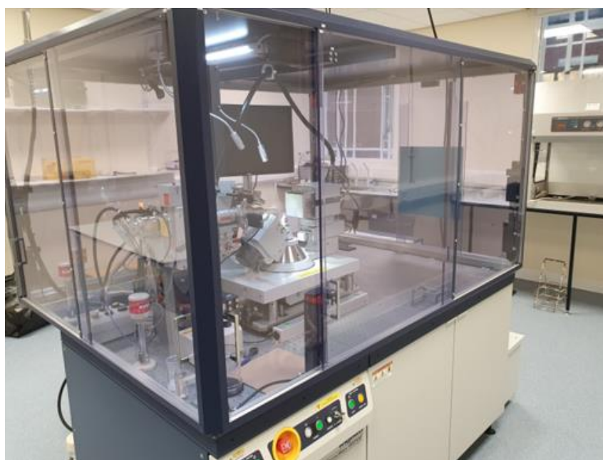
Figure 2.07: The X-ray enclosure of the Flow-XI lab-source X-ray instrument for in situ studies during crystallisation.
