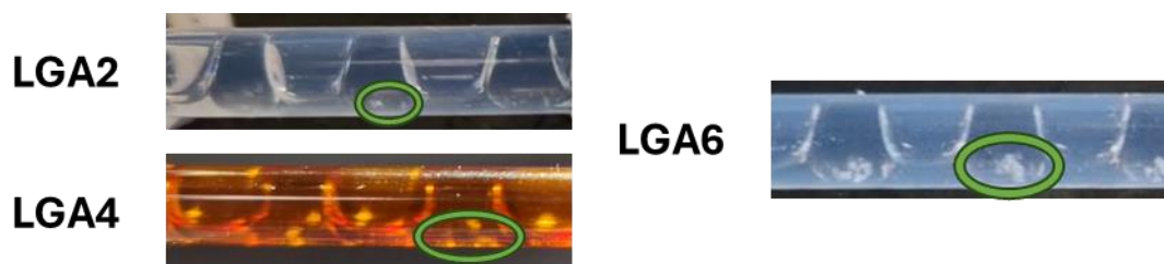
Figure 4.11: Images of the levels of crystallisation around the X3 region for LGA2, LGA4, and LGA6. Note: LGA4 showing the Kapton window tubing section.
