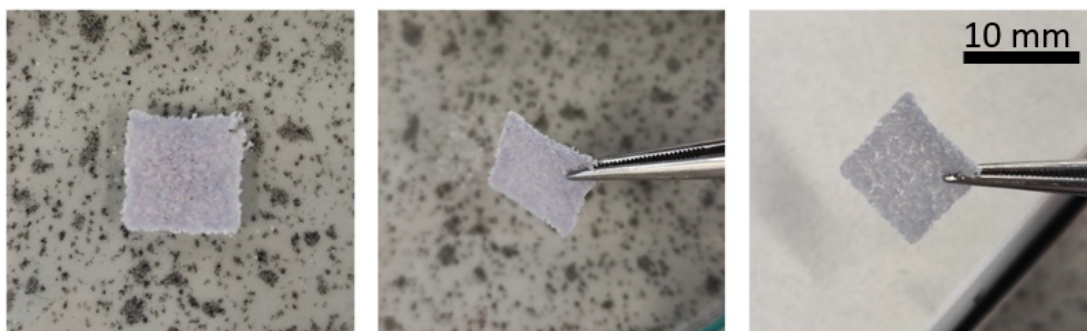
Figure 5.7: Image array of a fully consolidated single powder layer (SPL) sample of 0.82 \mu\text{m} thickness printed using binder system A01 – B102; A01 jetted at 35 V/60 °C and B102 jetted at 33 V/55 °C.
