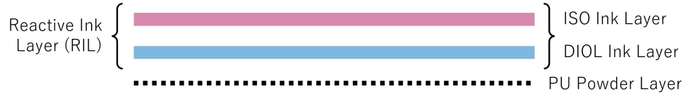
Figure 5.12: Composition of a single Reactive Ink Layer (RIL), totalling one DIOL ink layer and one ISO ink layer, in any deposition sequence.
