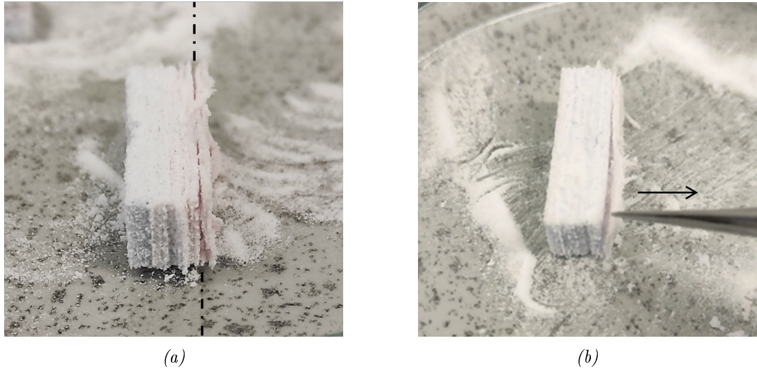
Figure 6.14: Rectangular 3D RBJ part built above a supportive raft where (a) highlights the boundary with the dotted line and (b) demonstrates how the raft is removed during post-processing.
