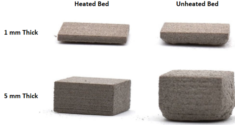
Figure 2.15: Comparison of geometric accuracies for unheated and heated BJ parts composed of single (1 mm) and multiple (5 mm) layers. 67
