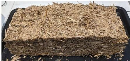
Figure 6-4 The effect of pasteurisation on the appearance of briquettes M2-4, compared to M1
