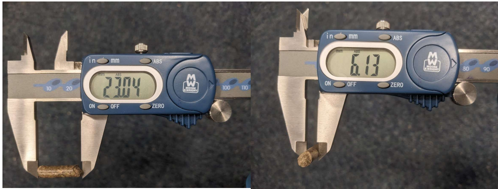
Figure 3-13 Measurement of pellet size - length (left) and diameter (right)
