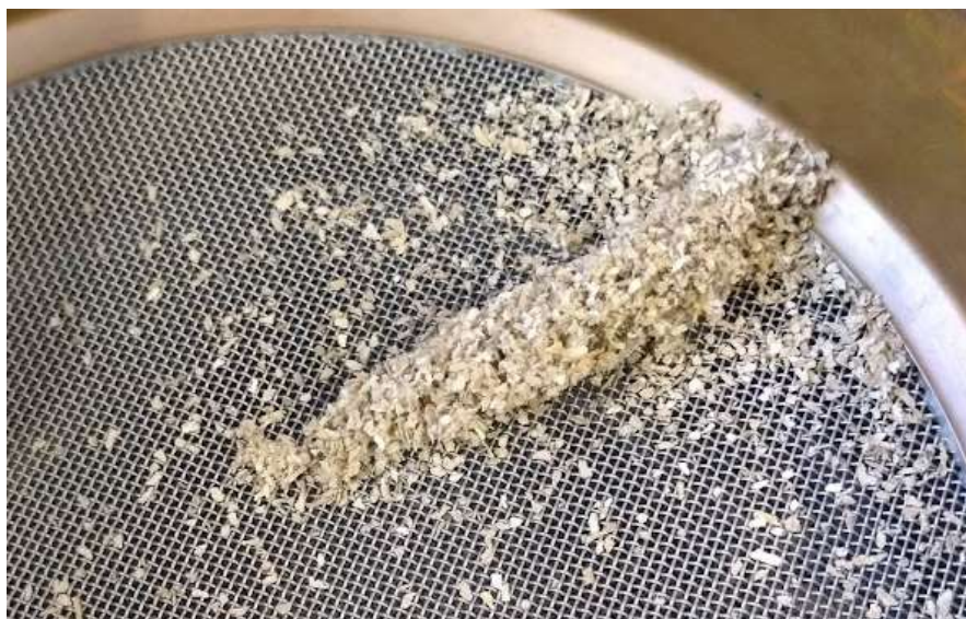
Figure 5-3 A ‘fluffy agglomeration’ of milled cardboard on a sieve
