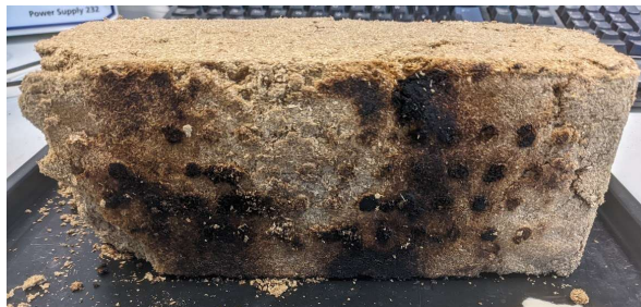
Figure 6-8 Charring on the bottom of briquettes SG7 immediately after pasteurisation
