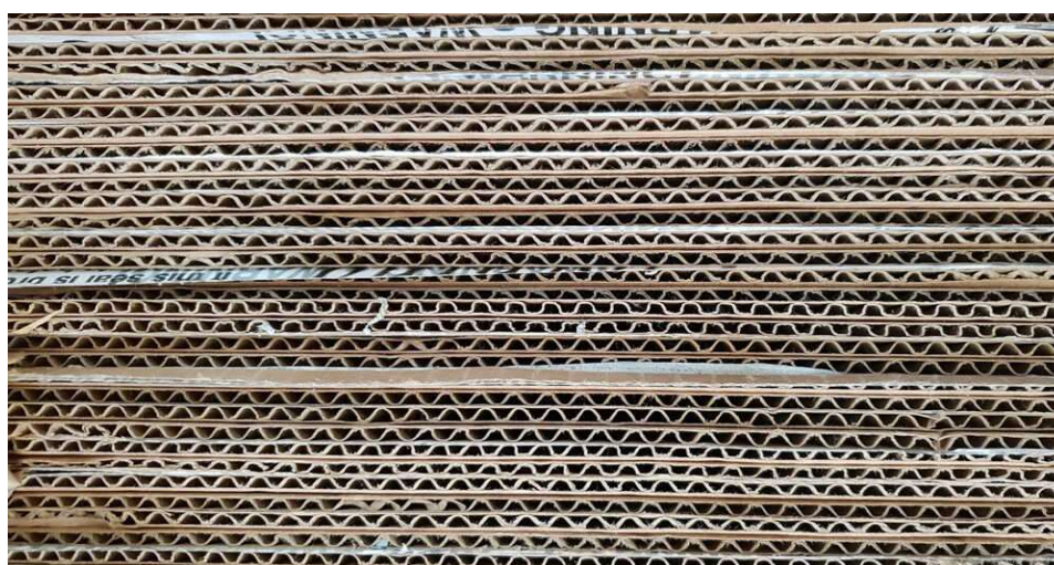
Figure 5-1 The structure of corrugated cardboard (Fruit Growers Supply, 2020)
