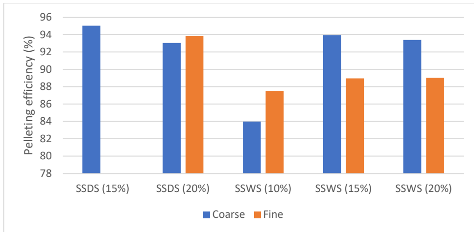
Figure 7-12 Influence of particle size on pelleting efficiency
