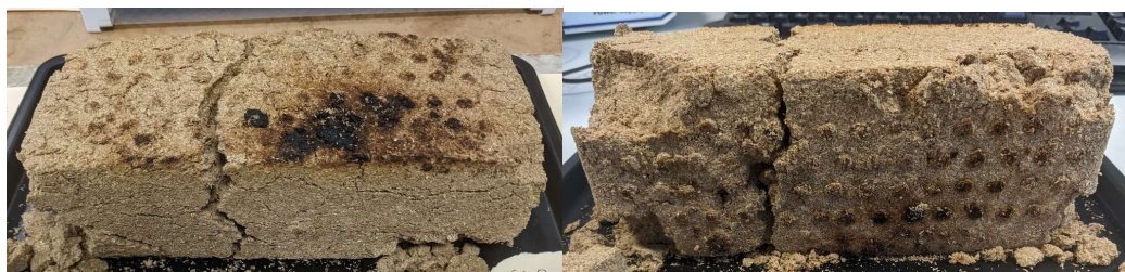
Figure 6-9 Charring on the top (left image) and bottom (right image) of briquette SG8 immediately after pasteurisation
