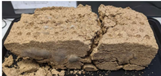
Figure 6-2 Briquette SG3 on day six of storage, with visible fungal growth
