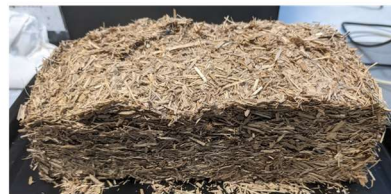
Figure 6-5 The effect of pasteurisation on the appearance of briquettes M6-8, compared to M5
