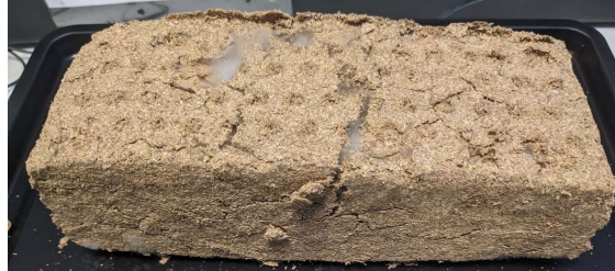
Figure 6-3 Briquette SG4 on day six of storage, with visible fungal growth
