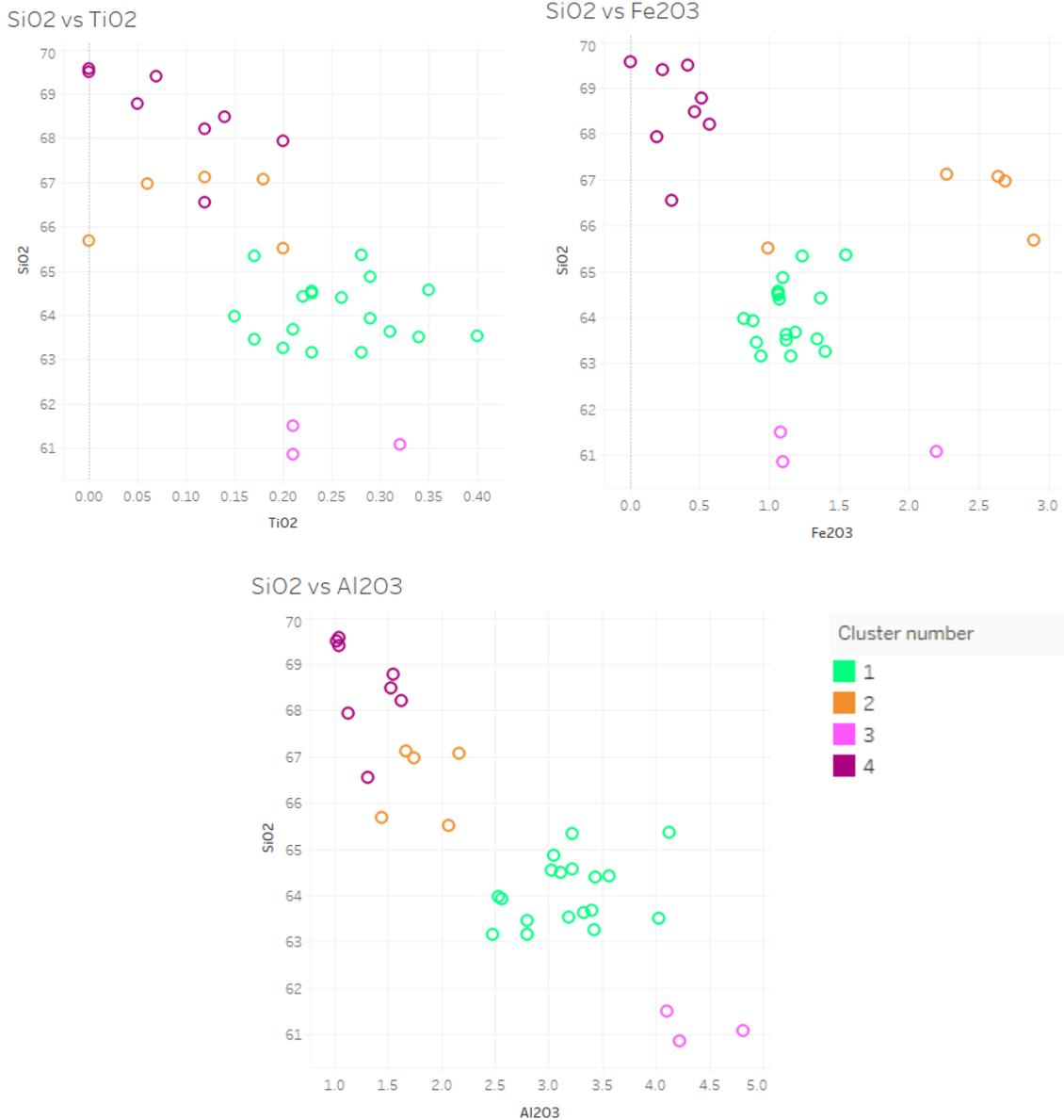
Figure 31a: (top left) biplot comparing the level of SiO<sub>2</sub> with TiO<sub>2</sub> across Clusters 1-4, b: (top right) biplot comparing the level of SiO<sub>2</sub> with Fe<sub>2</sub>O<sub>3</sub> across Clusters 1-4, c: (bottom) biplot comparing SiO<sub>2</sub> with Al<sub>2</sub>O<sub>3</sub> alumina across Clusters 1-4 (images produced by author using Tableau).
