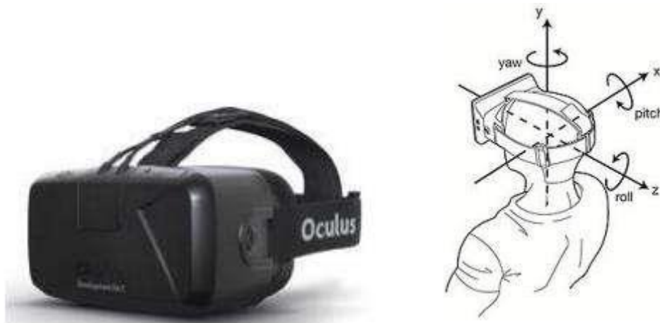
Figure 5: Oculus Rift visor (left), the rotation of Oculus Rift (right) (Goradia, Doshi & Kurup, 2014)
