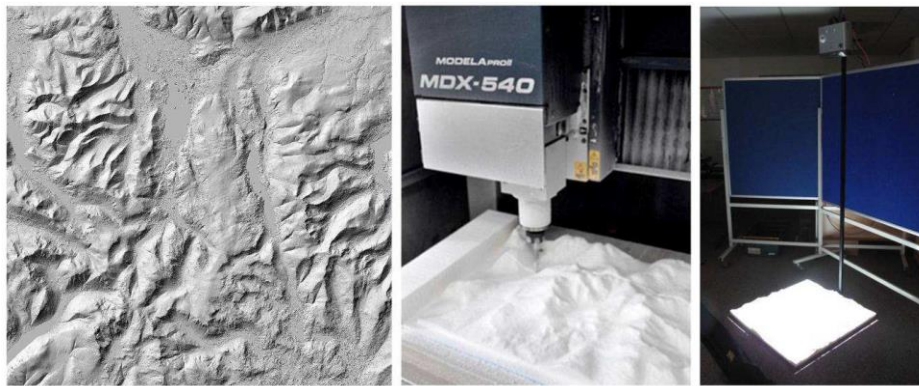
Figure 6: Creating the PARM prototype: Hillshade view of the DSM of Cumbria (left); The milling of one tile (centre); The prototype PARM system (right) (Priestnall et al., 2012).
