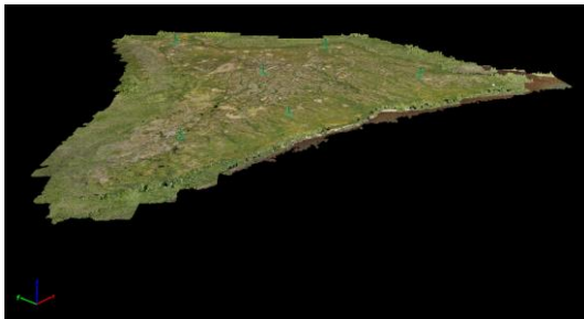
Figure 4. A processing image from Pix4D mapper of the Dense Point Cloud and ground control points (green and blue circle and arrows) for Voanjal.
