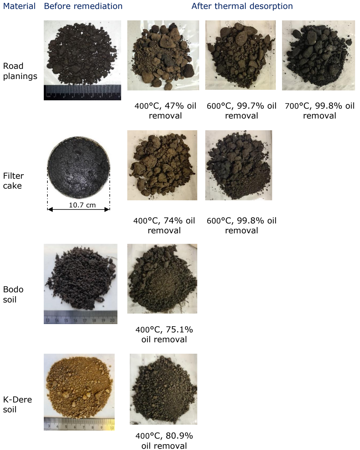
Figure 7-4: Thermal desorption of 20 g of hydrocarbon-contaminated materials at 30 minutes holding time. 1 L/min N 2 flow was used as a purge gas
