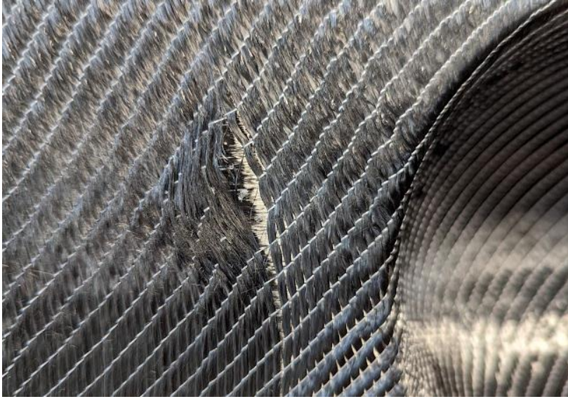
Figure 3.16 - Example of in-plane fibre distortion caused by anisotropic friction in the forming process.
