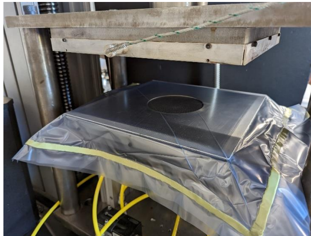
Figure 3.7 - Image of hemisphere forming test quadrant plates, in-situ of sealed diaphragms.
