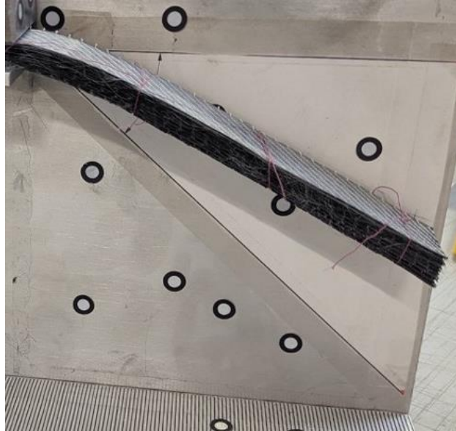
Figure 6.2 - A multi-ply bending sample of FCIM359. Pink loops of light-weight thread to prevent deconsolidation of the stack and reflective points used for the laser scanner can be seen.
