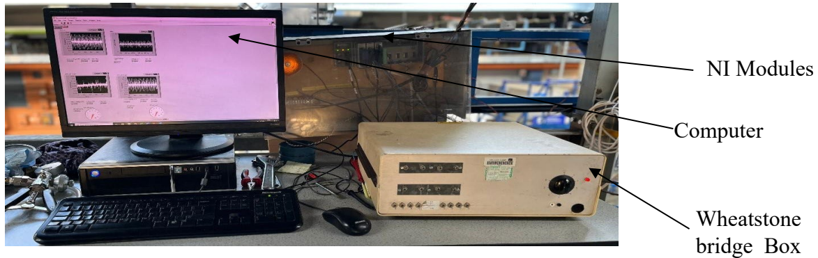
Figure 3.19: The data acquisition system comprising of the computer, NI modules and the electronic box.
