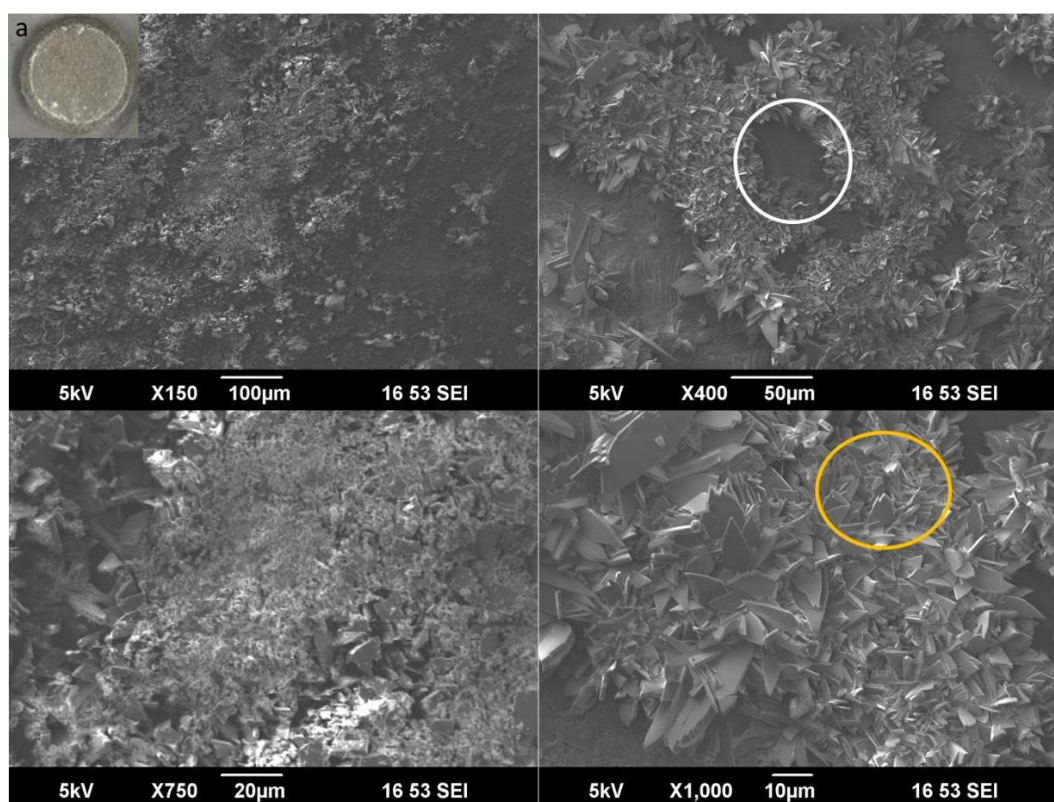
Figure 4.7: SEM images of electrodeposited CaP coating at 0.6 duty cycle showing increased coating coverage and decreased crystal size of needle-like structures (yellow circle) with typical coating voids (white circle) and a) a macroscopic image of the 0.6 duty cycle coating on Mg WE43 disc
