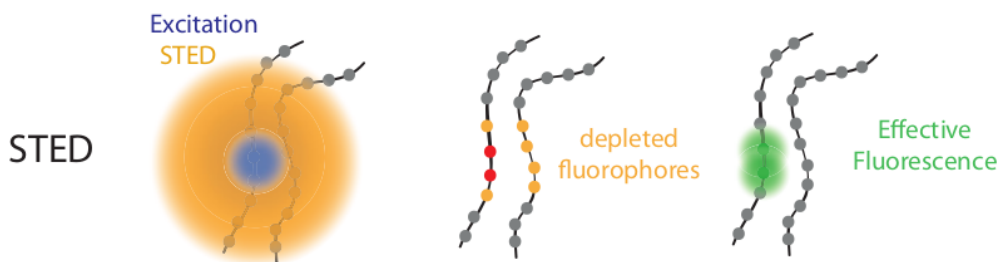
Figure 1.2: Enhancement of spatial resolution using STED microscopy. It depicts two wire-like entities marked with fluorophores represented by gray circles. The application of STED introduces a doughnut-shaped light pattern that intersects with the focal area's excitation spot. This interaction causes a depletion on most of the fluorophores within the doughnut area, denoted by yellow circles, effectively silencing their fluorescence. Consequently, only the central fluorophores within the doughnut emit fluorescence, indicated by a green glow, resulting in increased imaging resolution.
