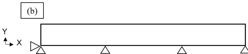
Figure 4.13: (a) shows the image of the CSAM sample holder, showing the mechanical constraint provided by the sample holder, and (b) shows a schematic illustration of the mechanical boundary conditions applied to the stress FEM.
