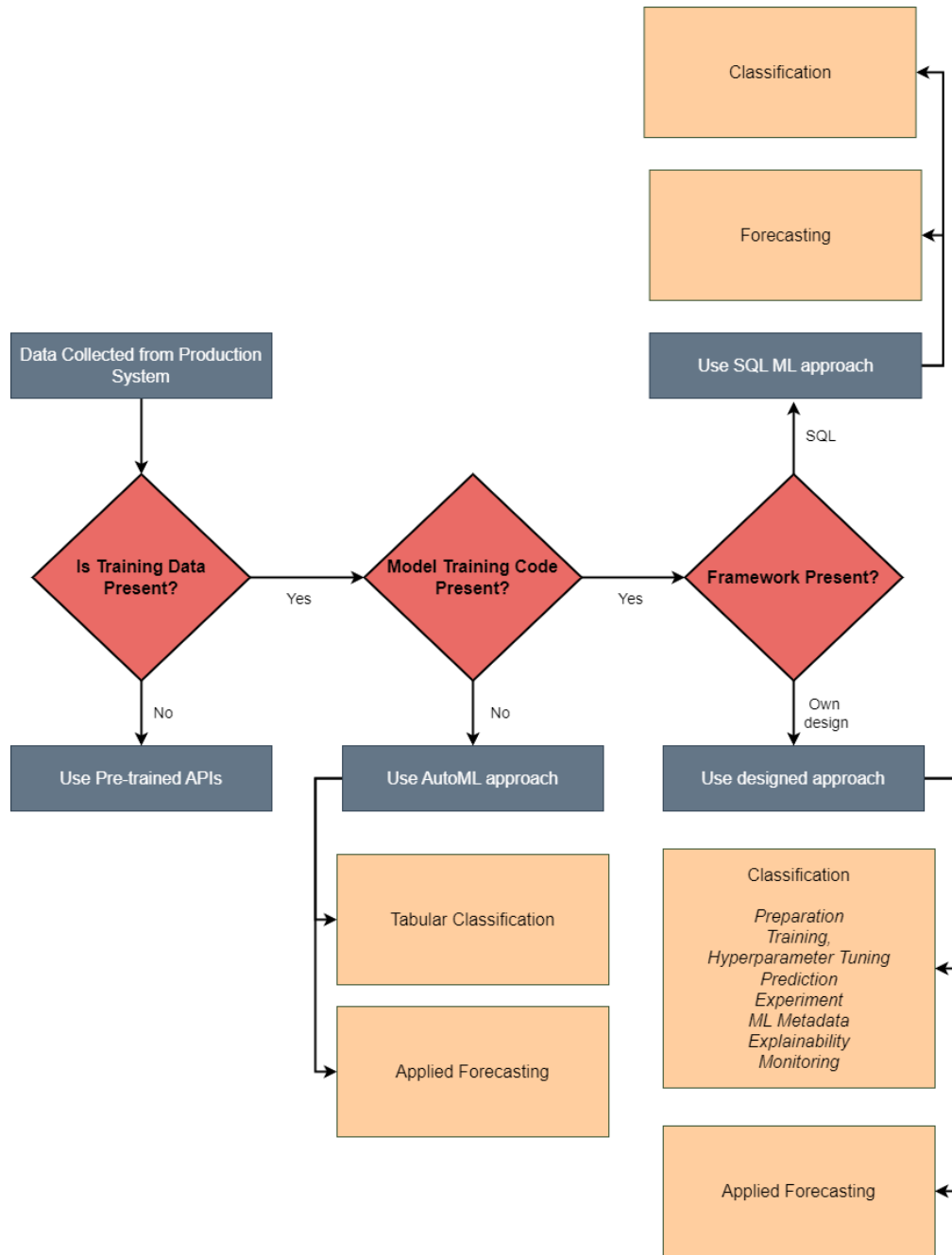
Figure 8.10: The generalised elaborative approach for predicting configuration values for configurable objects in production systems.
