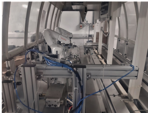
Figure 9.36: PRIME experimental setup involving teststation, two robots and a shuttle on rail.
