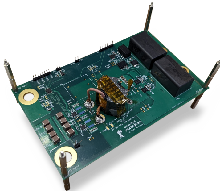
Figure 5.5: The converter PCB under testing.
