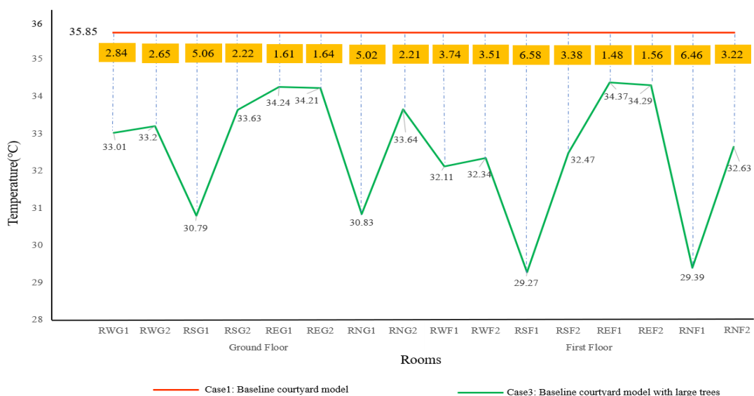
Figure 5.26 Comparison of air temperature for Case 1 and Case 3 in each room.
