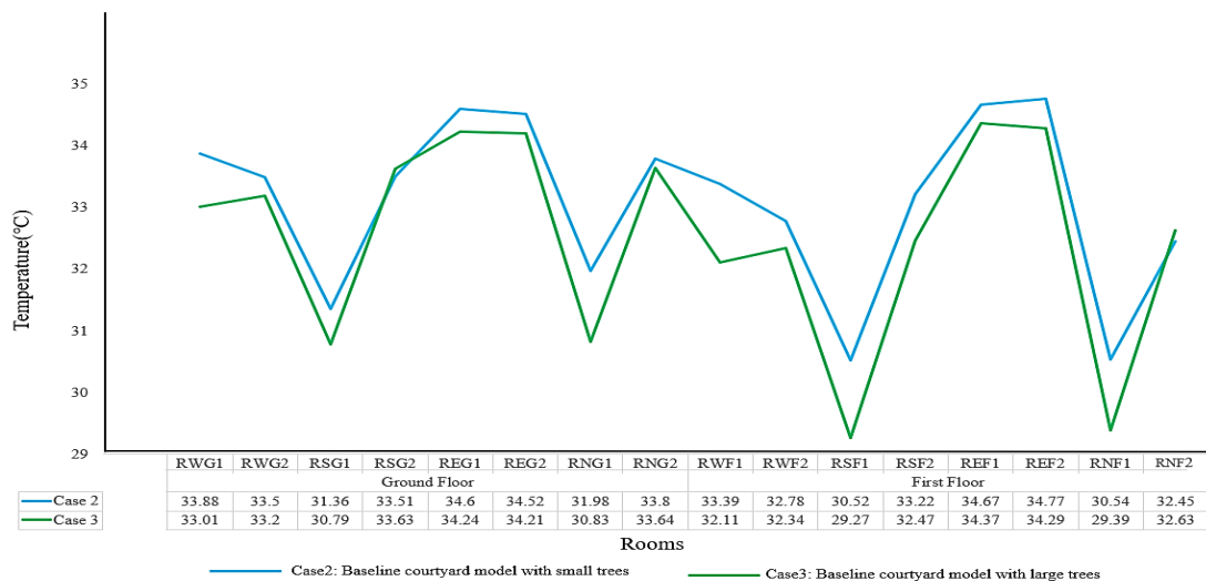
Figure 5.27 Comparison of air temperature for Case 2 and Case 3 in each room.
