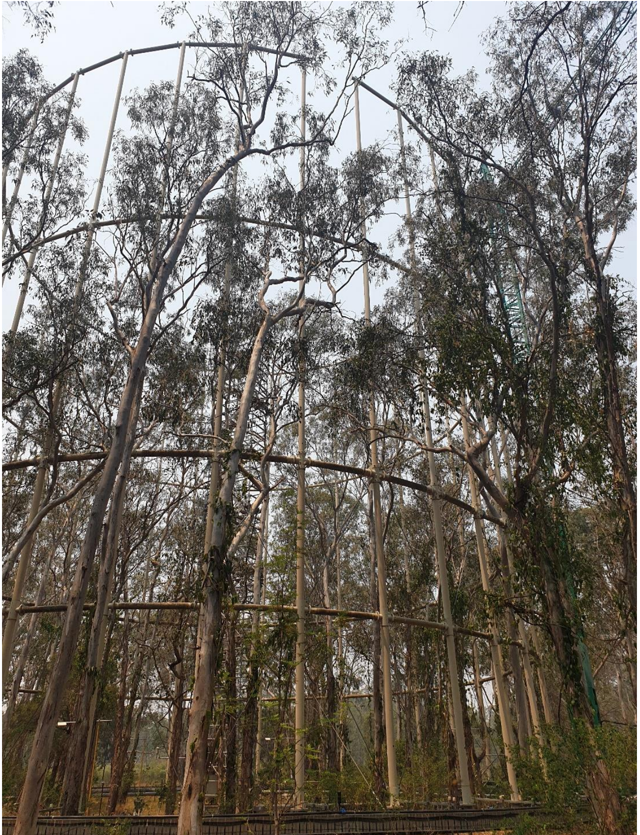
Figure 3. 2 EucFACE experimental ring. One of the 6 ring structures delivering CO 2 through 28m tall vertical vent pipes. Ring structure is 25m diameter with a permanent observation tower in the centre of the ring.
