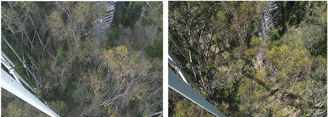
Figure 5. 1 Example of images from EucFACE. Left hand image example of flattest light for use in image amalgamation. Right hand image too bright for use in analysis. Bright images suffer from shadow occlusion of understory vegetation and typically non-linear sensor response to illumination. Both images show ring 6 (ambient) at EucFACE and are from 2021, November 11th for left image, January 16th for right image. Both images taken at 12pm facing south from 22m above ground level.
