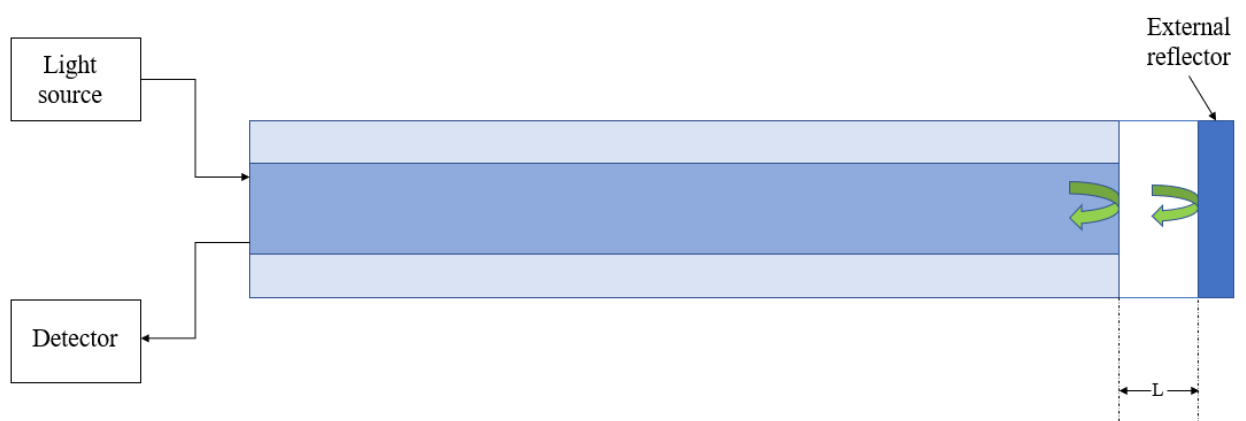
Figure 2- 19. A Fabry-Perot interferometer based in an optical fibre.
