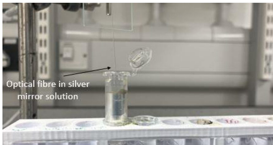
Figure 12. The deposition of silver film on the tip of optical fibre
