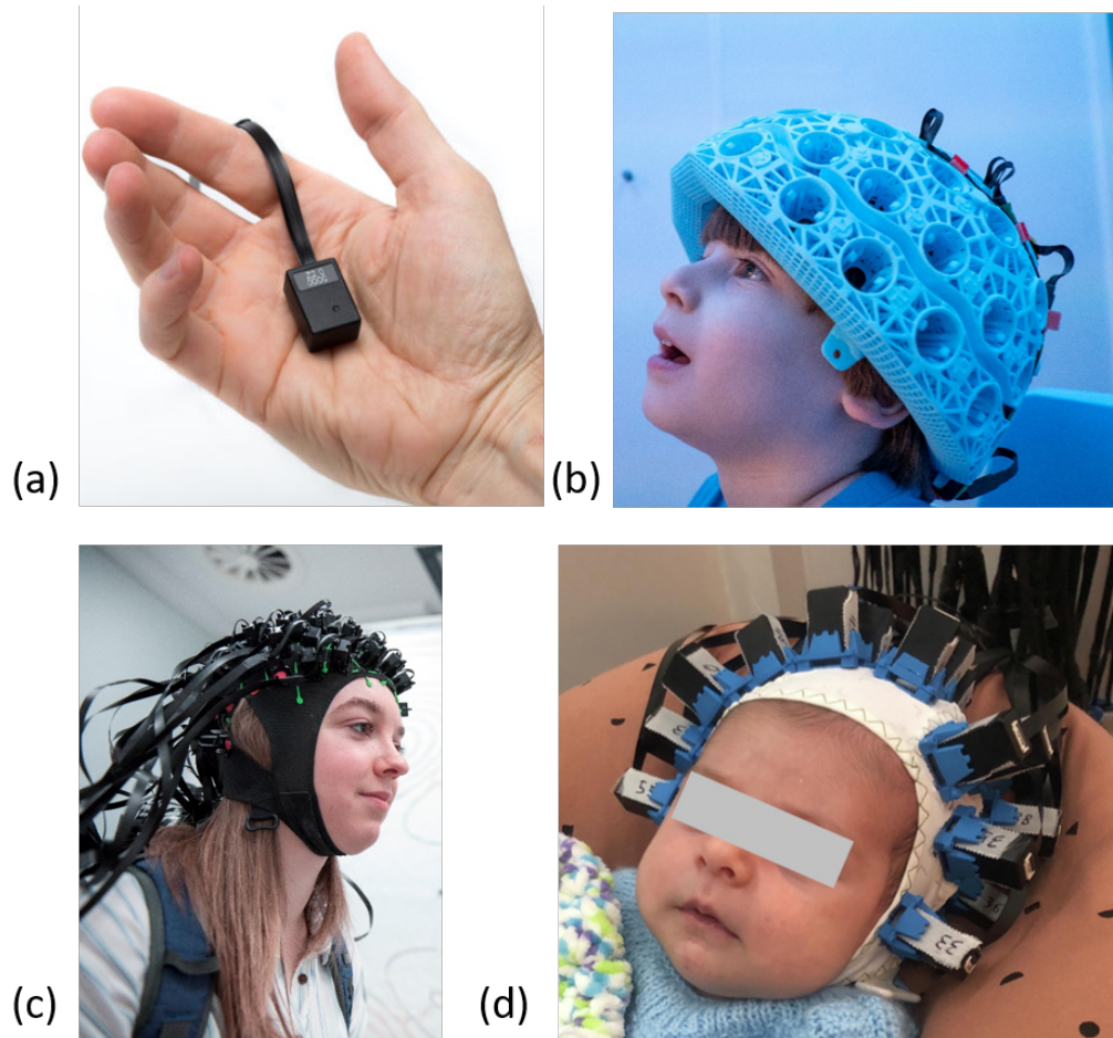
Figure 2.25: Photographs of an OPM and OPM-MEG helmets. (a) A QuSpin Zero-Field OPM Gen 2 (Photo courtesy of QuSpin Inc.). (b) A child-sized rigid OPM-MEG helmet (Photo courtesy of the University of Nottingham). (c) A flexible MEG cap (Photo courtesy of the University of Nottingham). (d) A baby wearing a flexible OPM-MEG cap (Taken from Feys et al. [2023]).
