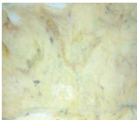
Figure 4-1: Surface morphology of the neat GP-22 sample heated at 260 °C for 10 minutes at rotor speed of 30 rpm
