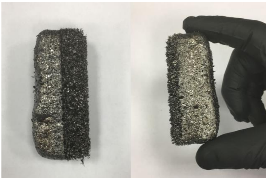
Figure 5.2. Photograph of the IL after carbonisation at 800 °C.
